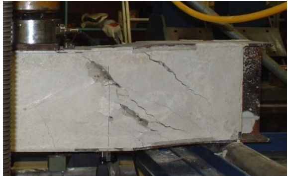
Figure 10. USFB No.4 at Failure point.
