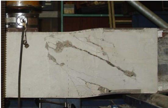
Figure 9. USFB No.3 at Failure point.
