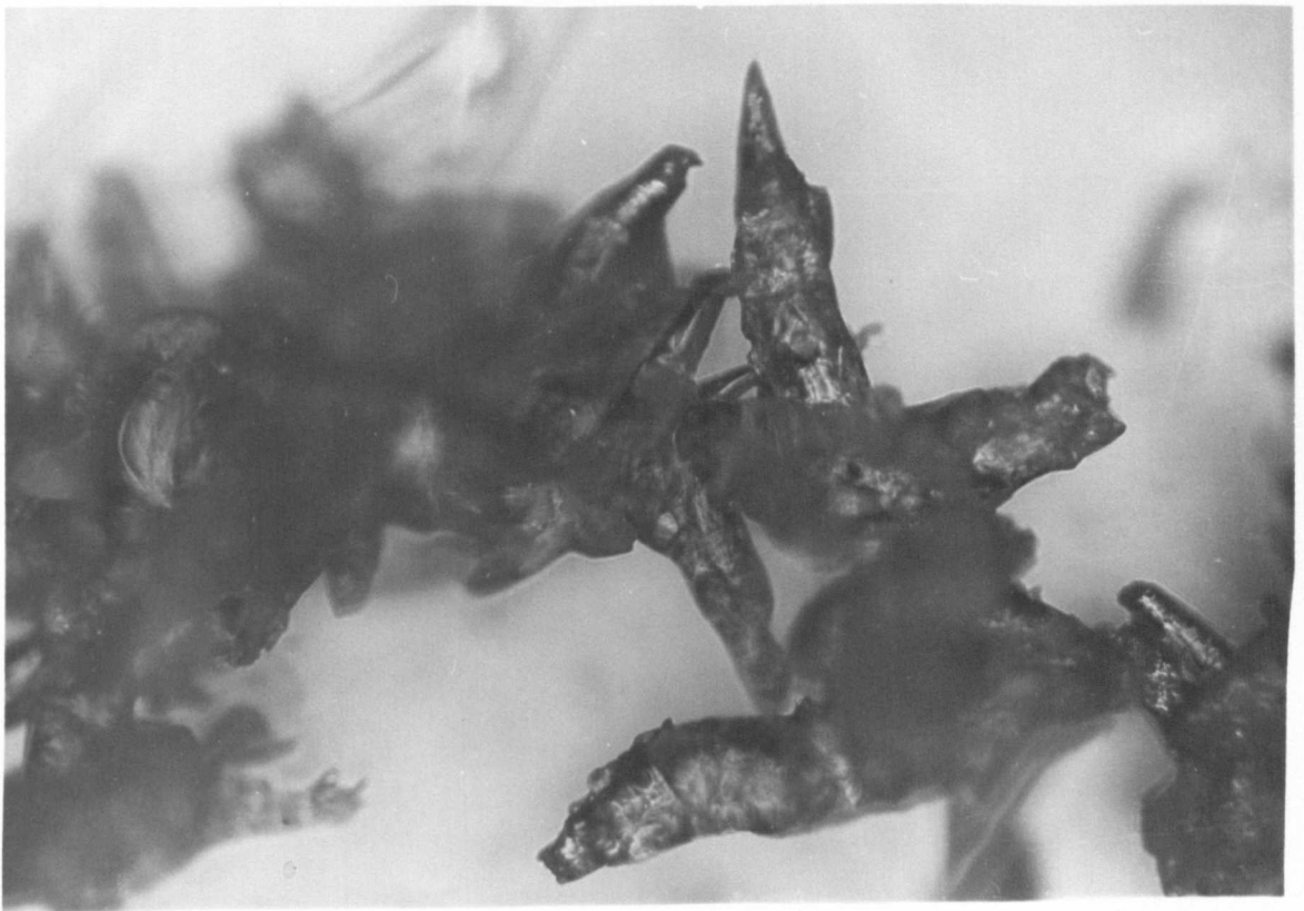
iii) paraffin wax crystals formed from a mixture of waxes ( x 450).
