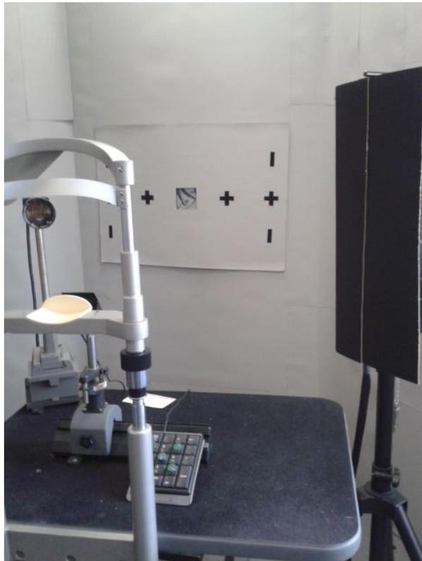
**Figure 46.** Experimental setup showing the display area, chin rest, and one of two illumination systems
