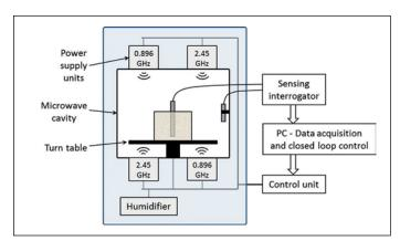
Figure 2: Schematic of smart microwave oven system.
