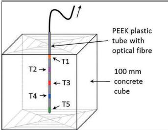
Figure 4: (a) Concrete cube in smart microwave oven at University College London. (b) Schematic of the five-point multiplexed FBG temperature probe developed at City University of London.
