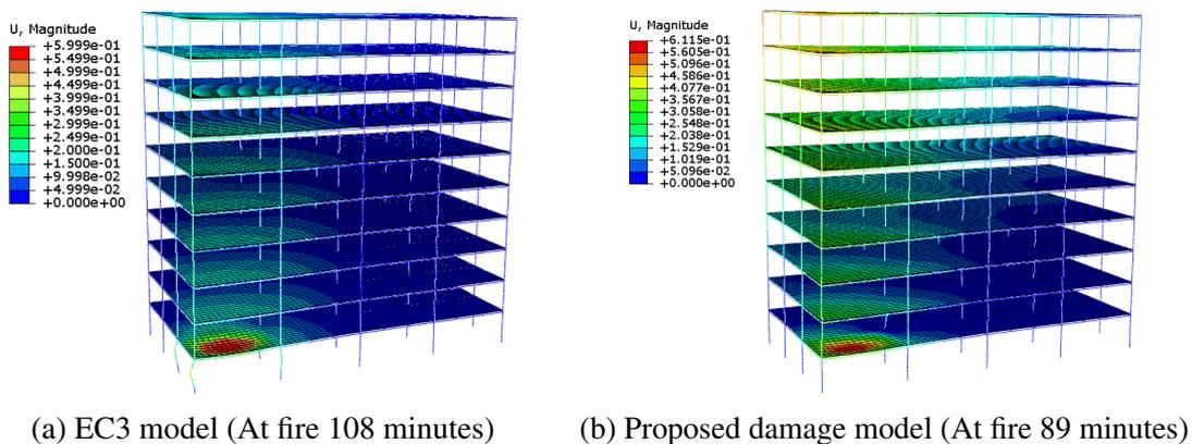
(a) EC3 model (At fire 108 minutes)      (b) Proposed damage model (At fire 89 minutes)
