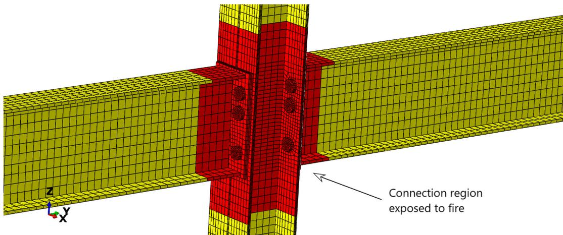
Fig. 4.14 Fire exposed region within connection model
