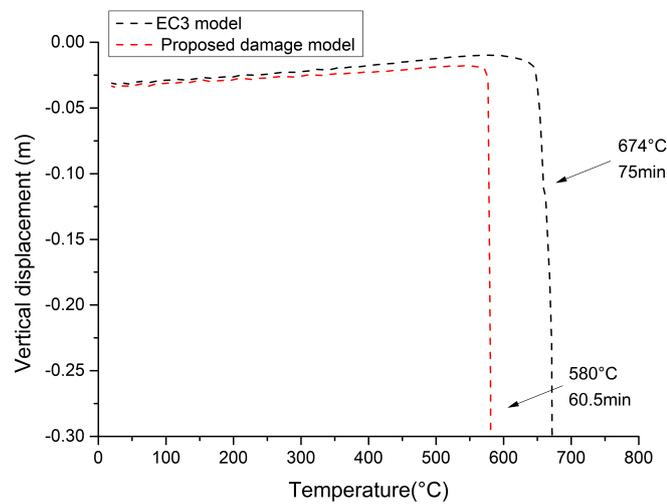
Fig. 5.68 Vertical displacement of the heated interior column B2
