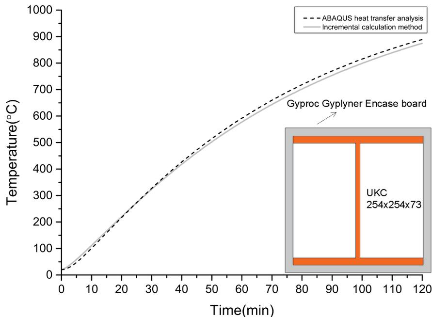
Fig. 5.3 Comparison of temperature histories of UKC254x254x73
