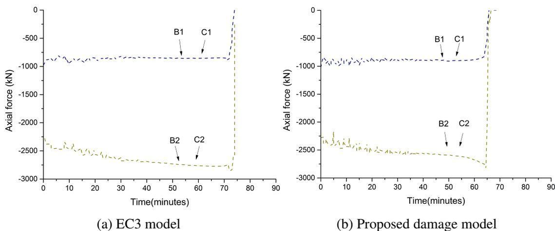
Fig. 5.59 Axial forces in columns during fire event
