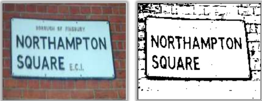
Figure 2-10: Pattern recognition of road signs a) Original image and b) Detected image
