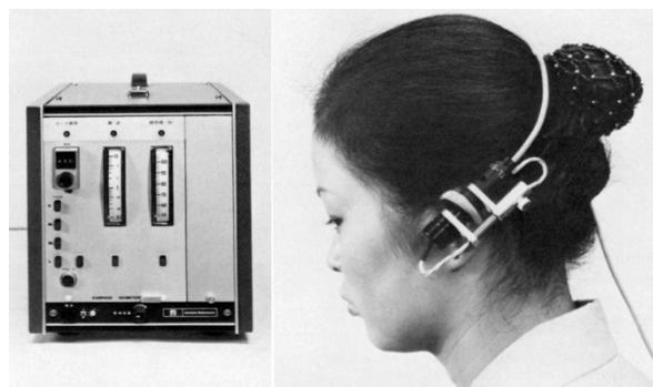
*Figure 4.5. The Nihon Kohden OLV-5100, the first commercially available pulse oximeter, with ear-probe (Aoyagi, 2003).*
