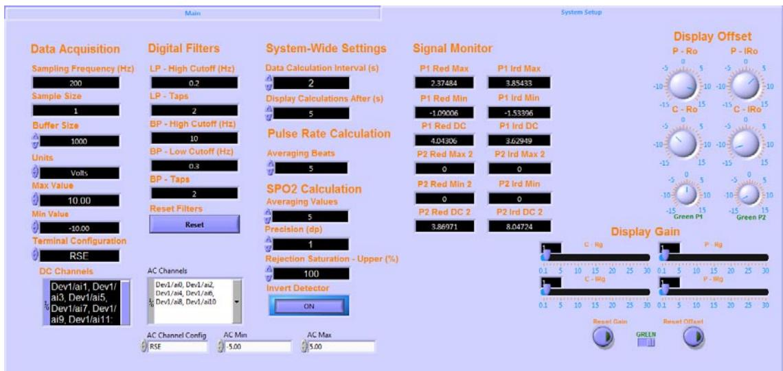
Figure 8.14b Virtual instrument UI front panel setup tab.
