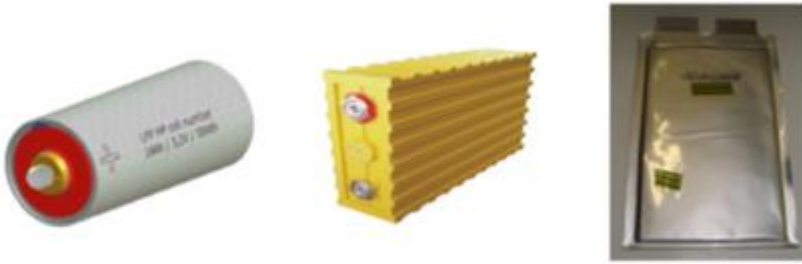
Figure 3: Cell designs (Cylindrical, Prismatic and Pouch) [4]
