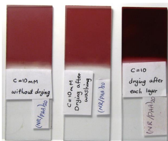
Fig 4-19 Comparison the glass slides coated by (NR/PAA) 20 at three different drying conditions: without drying, drying after washing, drying after each stage.
