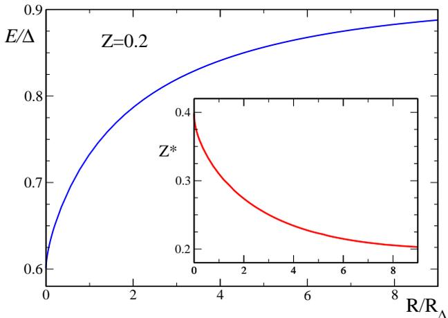
**Fig. 1.** Main panel: LCAO result for the ground-state energy,  $E$ , vs impurity distance  $R$  (which is given in units of  $R_\Delta = \hbar v_F/\Delta$ ), for the two-center potential with  $Z_1 = Z_2 = Z = 0.2$ . Inset: Optimal choice for the variational parameter,  $Z_{\text{eff}} = Z^*$ , determining the LCAO ground state, as a function of  $R$ .
