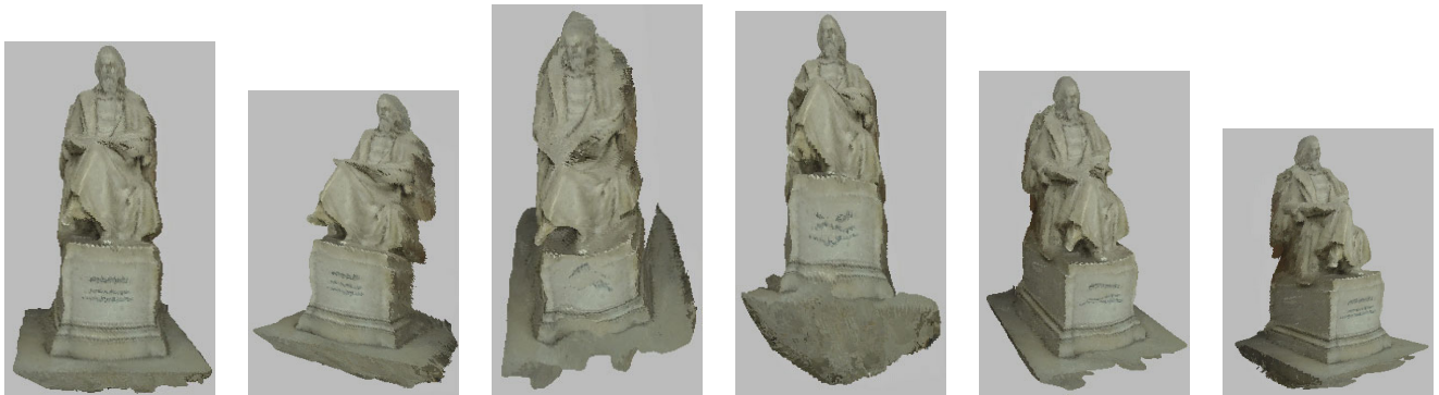
Figure 2. Reconstruction of Lord Tennyson statue. The top row shows two of the input images followed by views of the initial and final surface. The bottom row shows many more views of the final reconstruction with texture mapping of the original image data.
