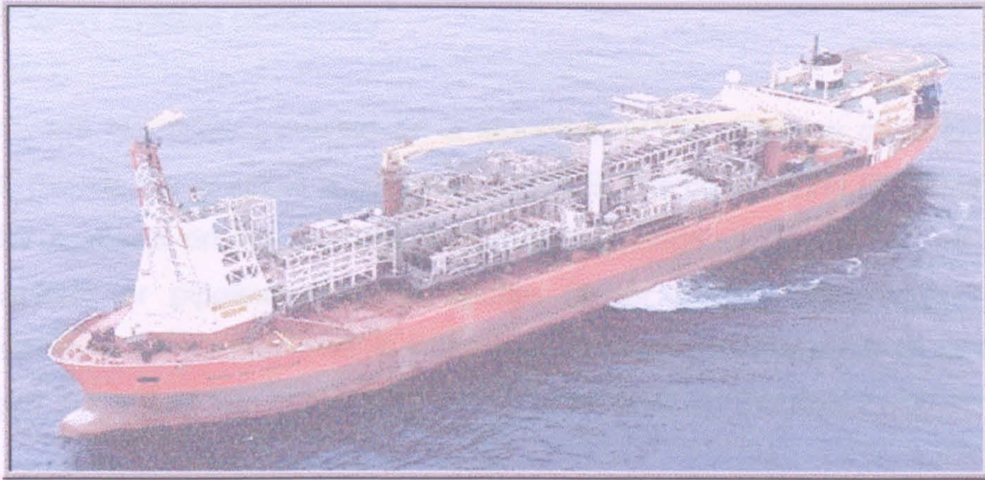
Figure 2-17 Upwind Flaring System on the Curlew FPSO (Courtesy of Maersk)
