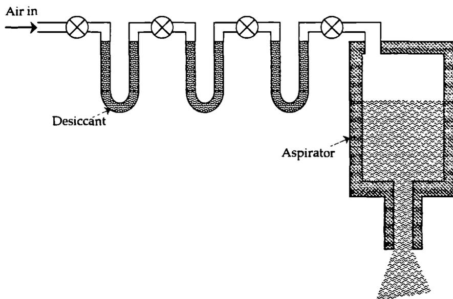
**Figure 12** Principle of early gravimetric or "chemical" hygrometer
