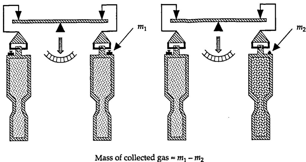
Figure 10 Illustration of complementary weighing of collected dry gas
