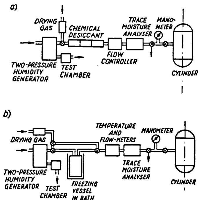
Figure 14 Block diagram of the gravimetric hygrometer of Poland (a) with chemical desiccant and (b) with cold trap (Kostyrko, 1979)
