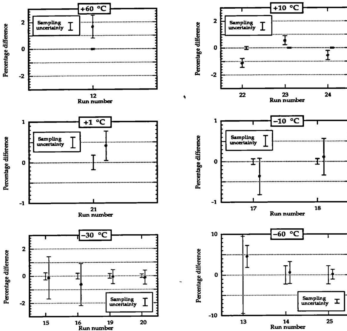
Figure 25 Graphs showing the results of measurements intercomparing the gravimetric hygrometer and NPL humidity generator.
