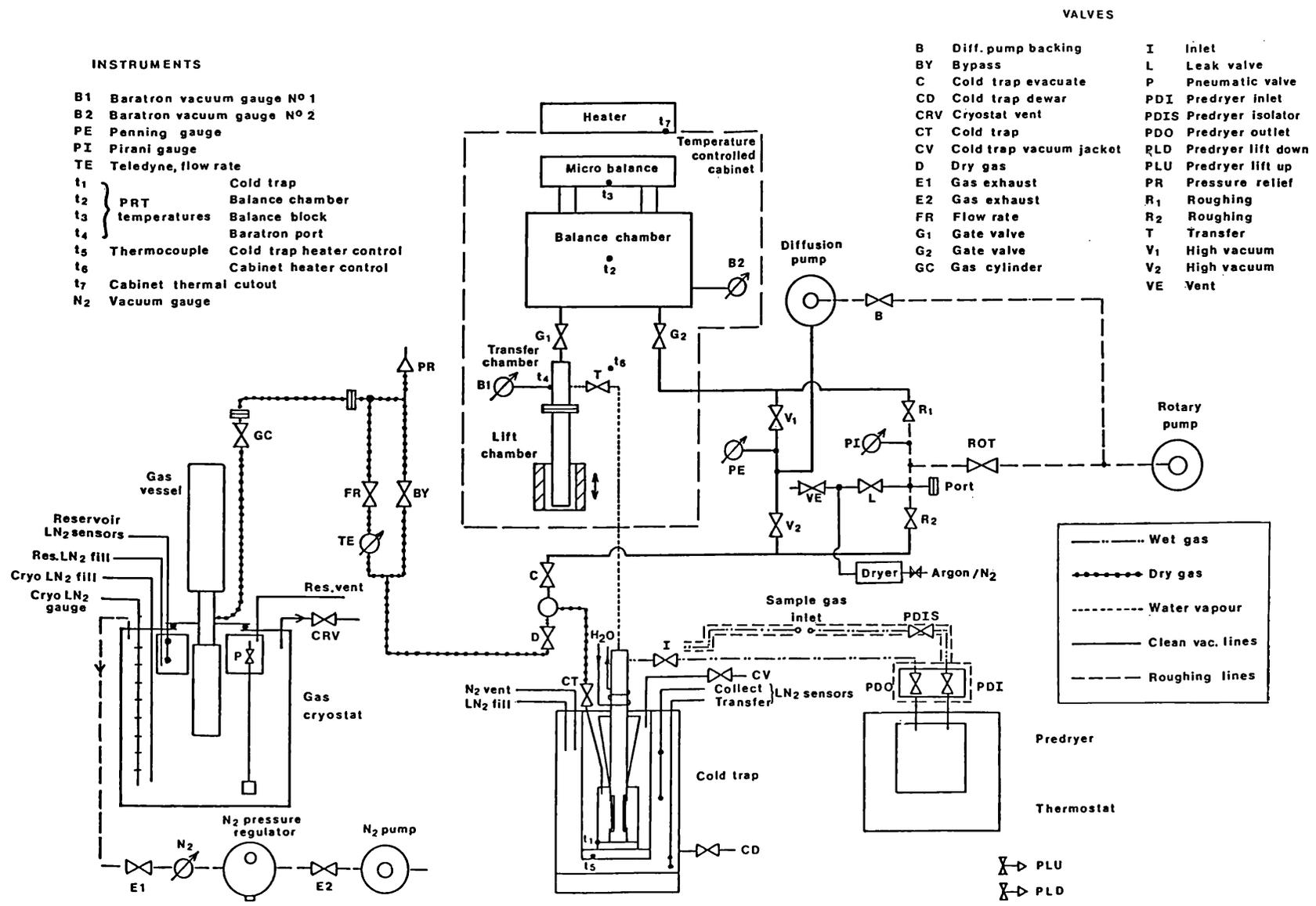
Figure 8 Detailed schematic diagram of the NPL gravimetric hygrometer (Sira Ltd, 1985)
