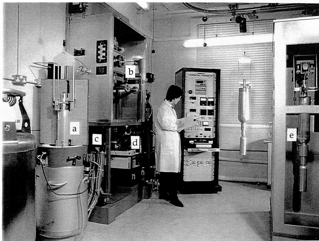
Figure 4 Photograph of the gravimetric hygrometer, showing (a) gas vessel in cryostat, (b) microbalance vacuum chamber, (c) cold trap, (d) predryer and thermostatted bath, and (e) gas vessel on equal-arm balance
