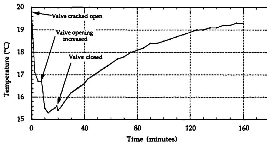
Figure 17 Graph of surface temperature of gas collection vessel during and after venting of enclosed gas to atmosphere
