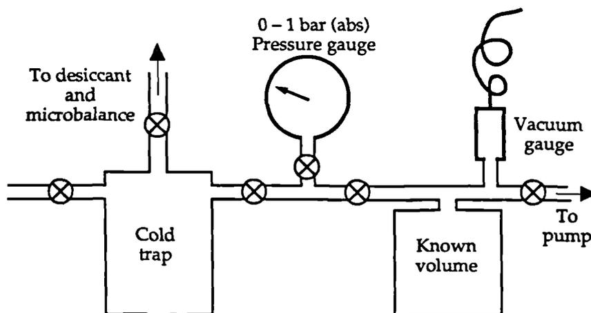
**Figure 21** Block diagram of experimental configuration used to evaluate the mass of gas trapped in the cold trap
