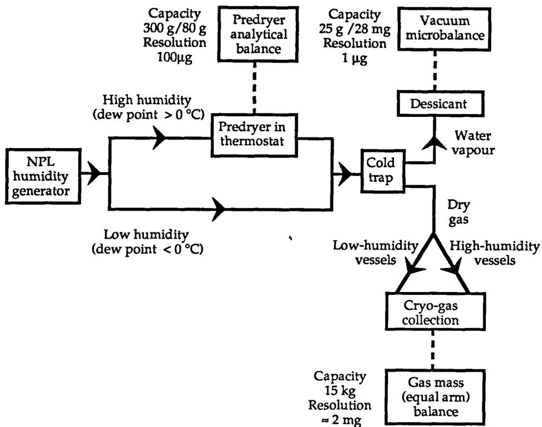
Figure 3 Block diagram of the gravimetric hygrometer
