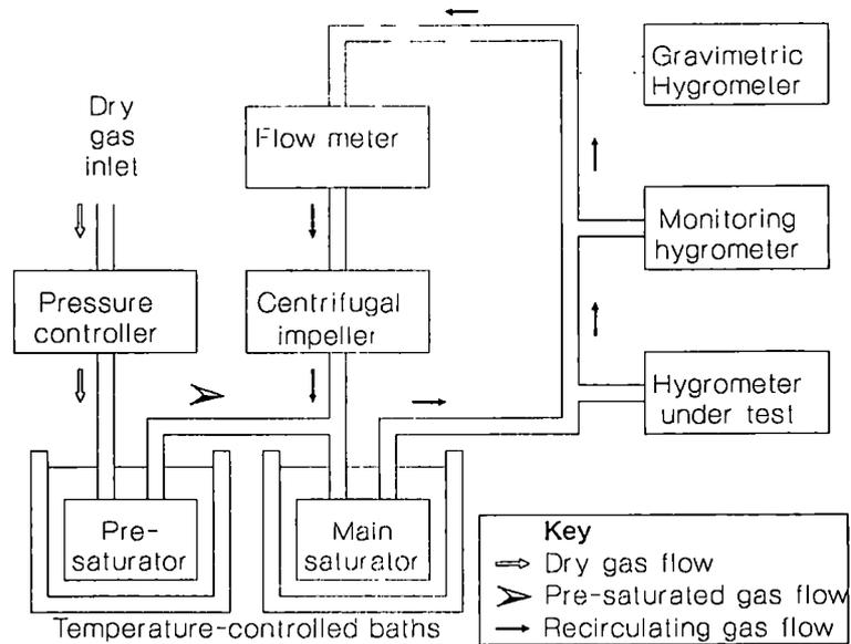
Figure 5 Block diagram of the NPL humidity generator
