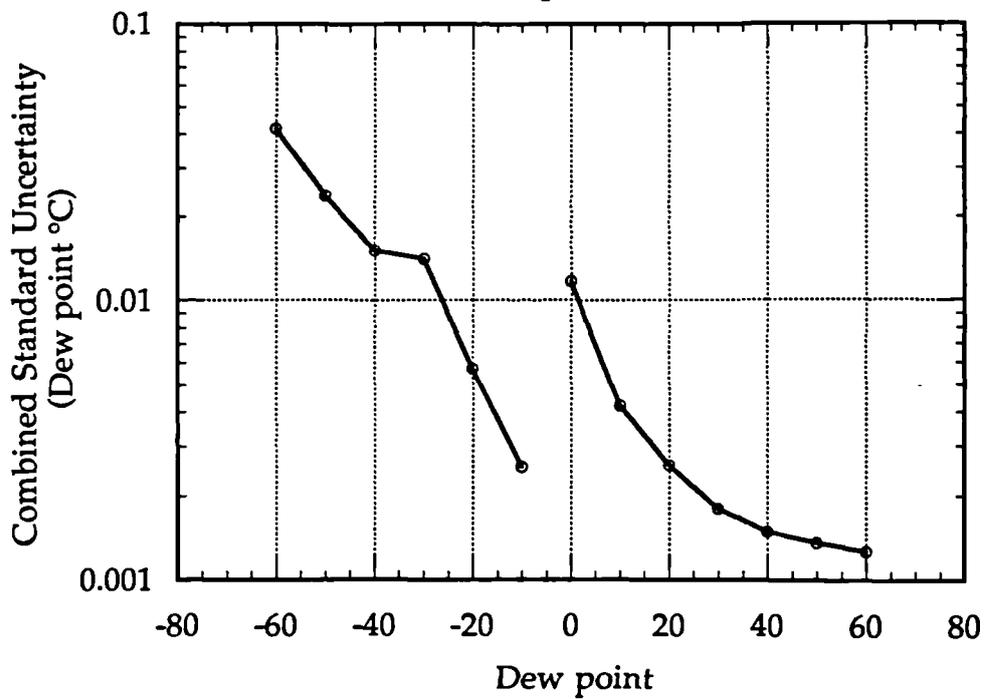
Figure 22 Combined standard uncertainty for gravimetric hygrometer (a) as a percentage of result (b) in dew-point equivalent
