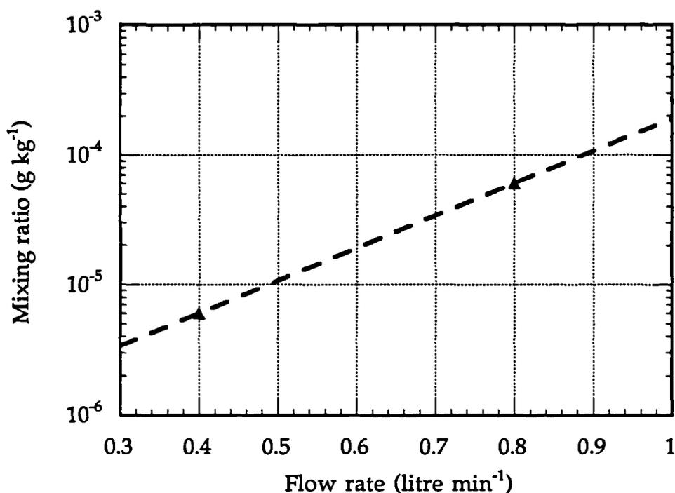
Figure 20 Graph showing estimated moisture content of exhaust gas from cold trap as a function of flow rate.
