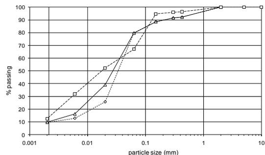
Figure 1. Typical particle size distribution curves for the unremoulded bulk sample
