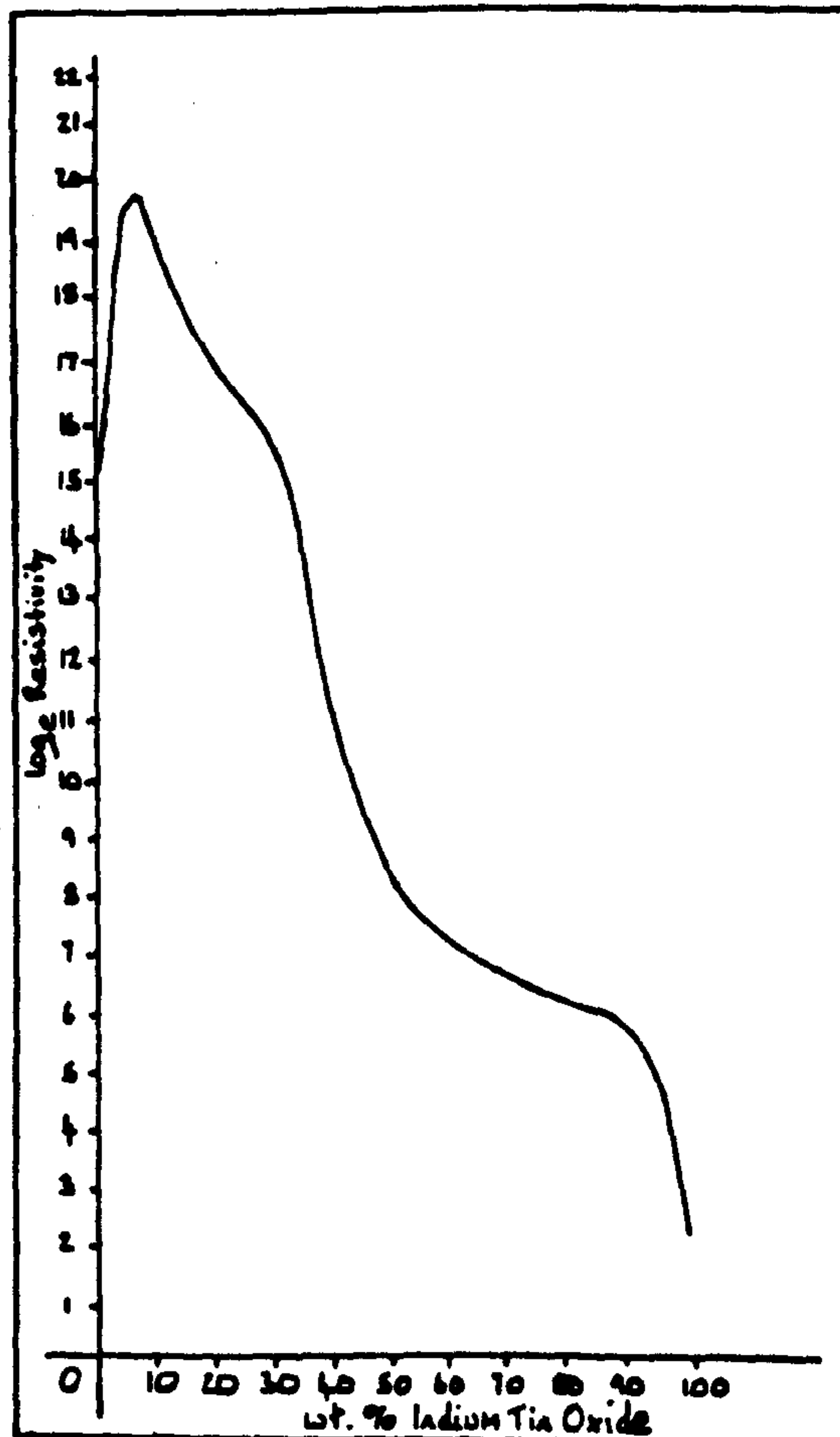
Figure Eight - log Resistivity v. Composition of Cryolite/In Sn Oxide Phases
