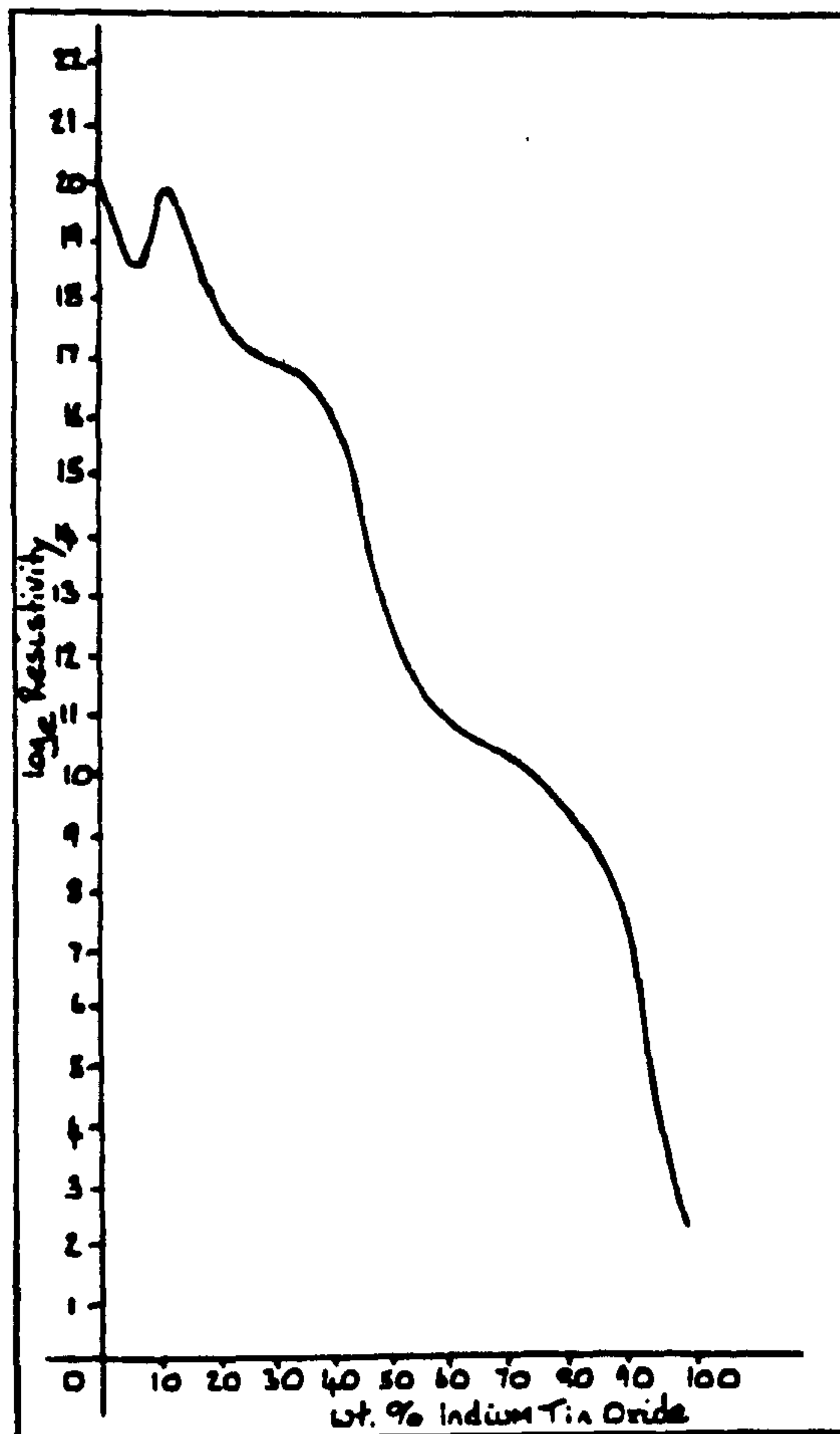
Figure Eleven - \log_e Resistivity v. Composition of Talc/In Sn Oxide Phases
