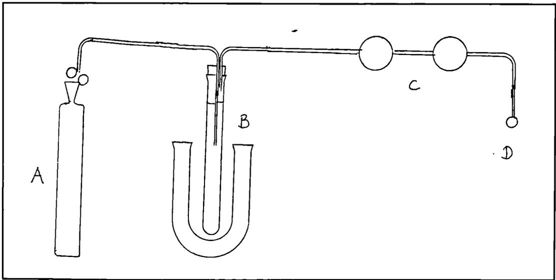
**Figure 3:3** A schematic representation of the experimental system used for  $H_2S$  and  $SO_2$  determination.
