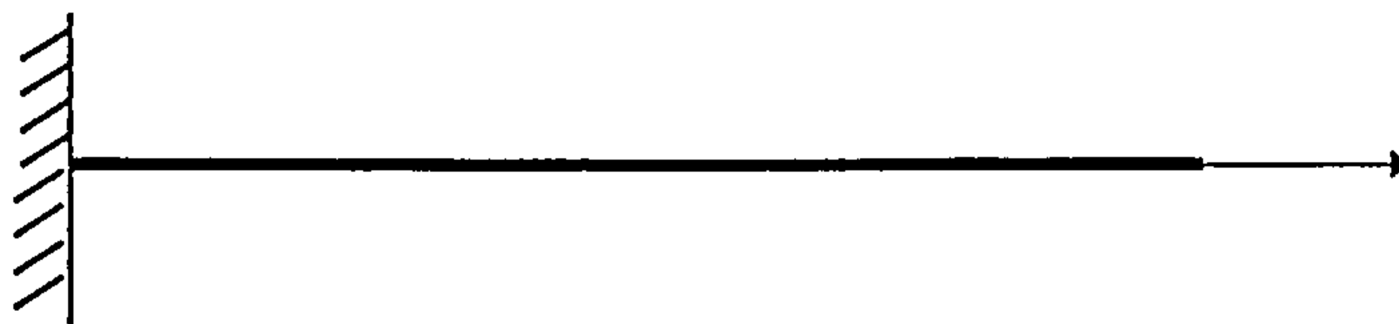
Fig 2-1: Tensile bar as energy absorbing device.
