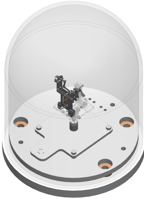
Figure 4.17: CAD of 0 Degree Inclination Vacuum Chamber Setup Iso View
