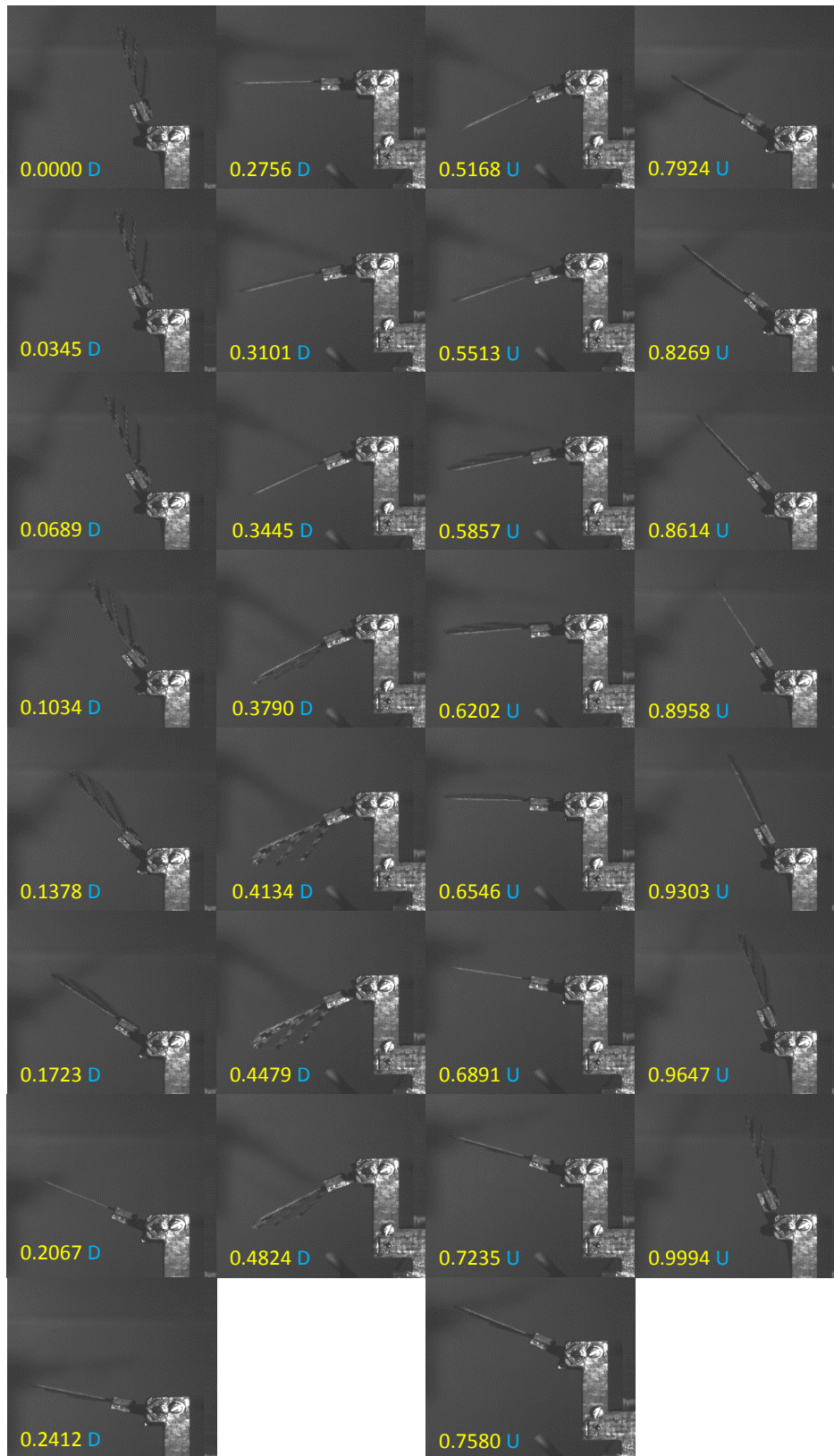
Figure 4.66: Wing Motion for 26 mm Semi-Rigid Wings (WT2) 75 microns 2 mm exposed flexible area, Vertical Stroke Plane, D: Downstroke and U: Upstroke
