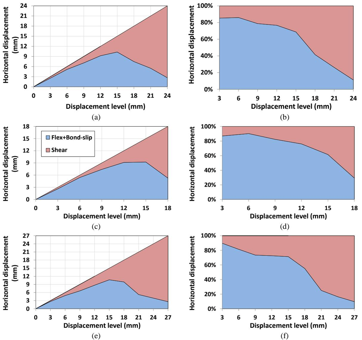
Figure 7-17: Lateral displacement decomposition for (a, b) SC<sub>1</sub>, (c, d) SC<sub>2</sub>, and (e, f) SC<sub>3</sub> in (left) absolute and (right) relative terms.
