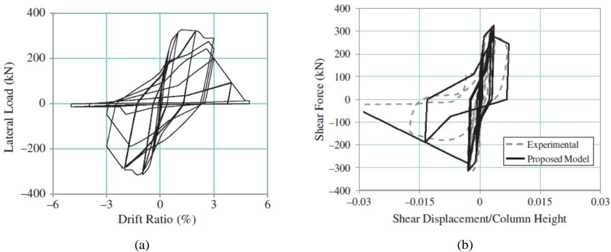
Figure 9-2: Comparison between the predicted response of Specimen-1 by the model proposed by Baradaran-Shoraka and Elwood (2013) and the experimental one in terms of (a) shear force against lateral drift ratio, (b) shear displacement over column height.
