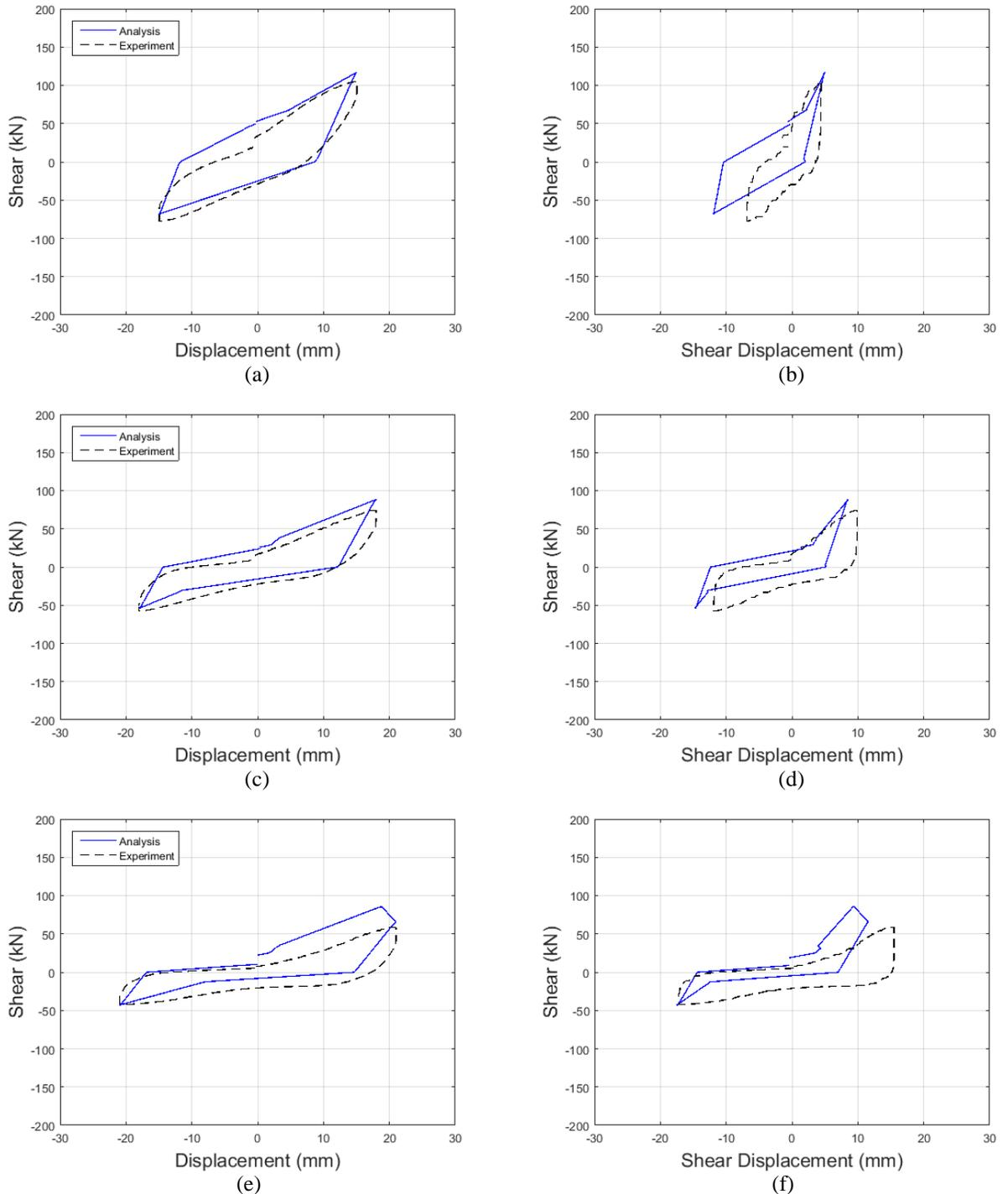
Figure 9-4: Comparison between individual cycles of the predicted response of FSC\_1 by the proposed model and the experimental one: (a, b) 3<sup>rd</sup> cycle at +/- 15 mm, (c, d) 2<sup>nd</sup> cycle at +/- 18 mm, and (e, f) 1<sup>st</sup> cycle at +/- 21 mm. (left) Total displacements and (right) shear displacements.
