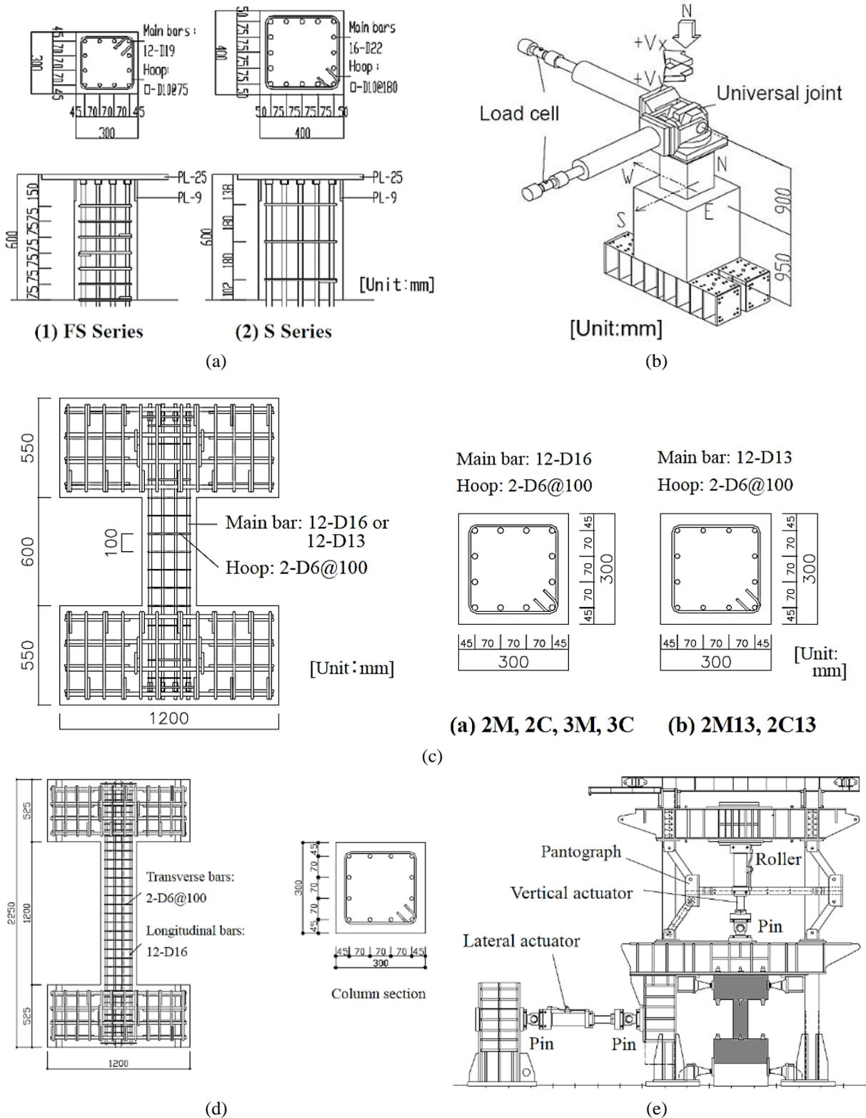
Figure 2-5: (a) Specimen design and (b) test set-up (Yoshimura & Yamanaka, 2000). (c) Specimen design (Yoshimura & Nakamura, 2002). (d) Design of specimen No. 1 (Yoshimura et al., 2003). (e) Test set-up (Nakamura & Yoshimura 2002).
