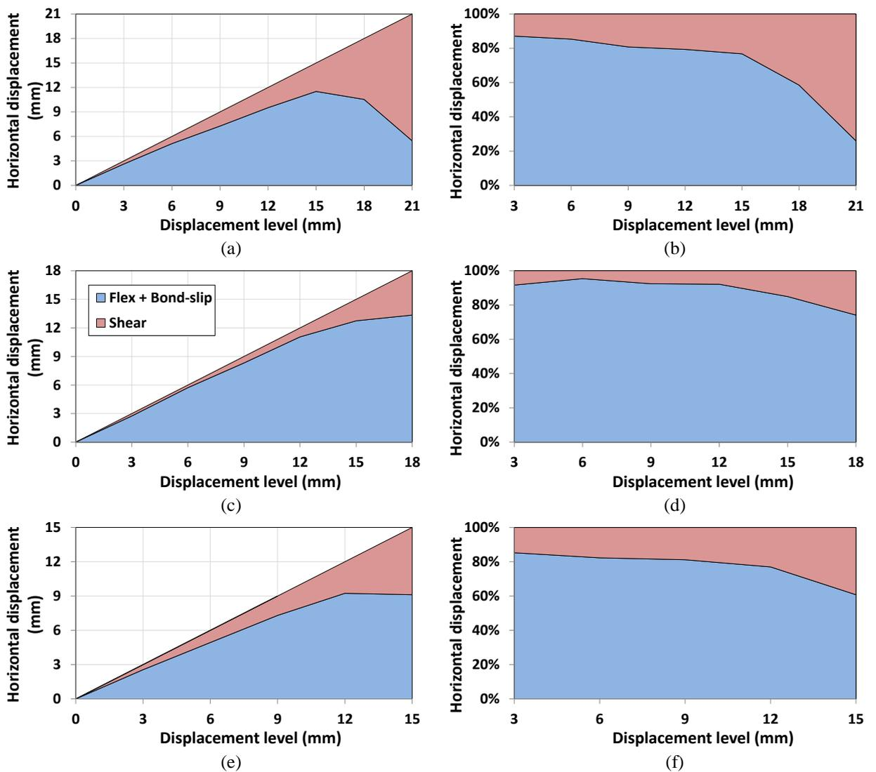
Figure 7-16: Lateral displacement decomposition for (a, b) FSC\_1, (c, d) FSC\_2, and (e, f) FSC\_3 in (left) absolute and (right) relative terms.
