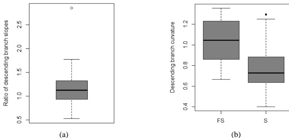
Figure 4-8: (a) Ratio of descending branch slopes in two “directions” of the response of the database specimens. (b) Curvature of the descending branch of the response of flexure-shear critical (FS) and shear critical (S) specimens of the database.
