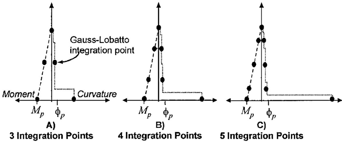
Figure 2-15: Numerical localisation in force-based elements in the case of softening response. (Coleman & Spacone, 2001)
