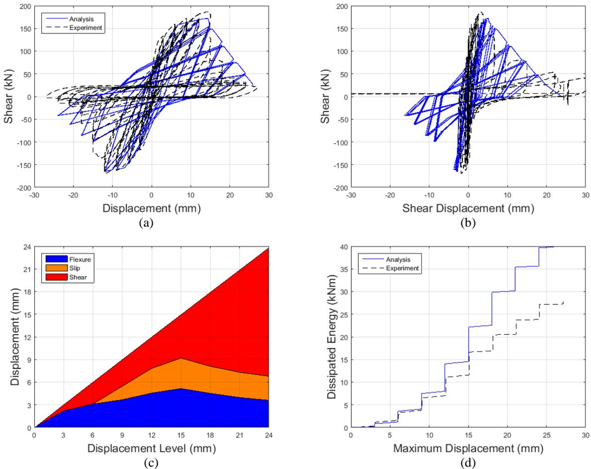
Figure 9-23: Comparison between the predicted response of SC\_3 by the proposed model and the experimental one in terms of (a) shear force against lateral displacement, and (b) shear displacement. (c) Decomposition of the element's lateral displacement components throughout the analysis. (d) Comparison between predicted and experimental cumulative dissipated energy.
