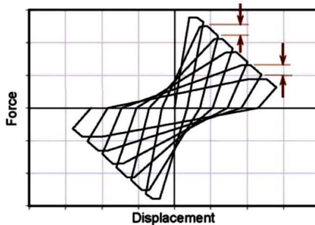
Figure 2-22: Example of in-cycle strength degradation. (ATC, 2009)
