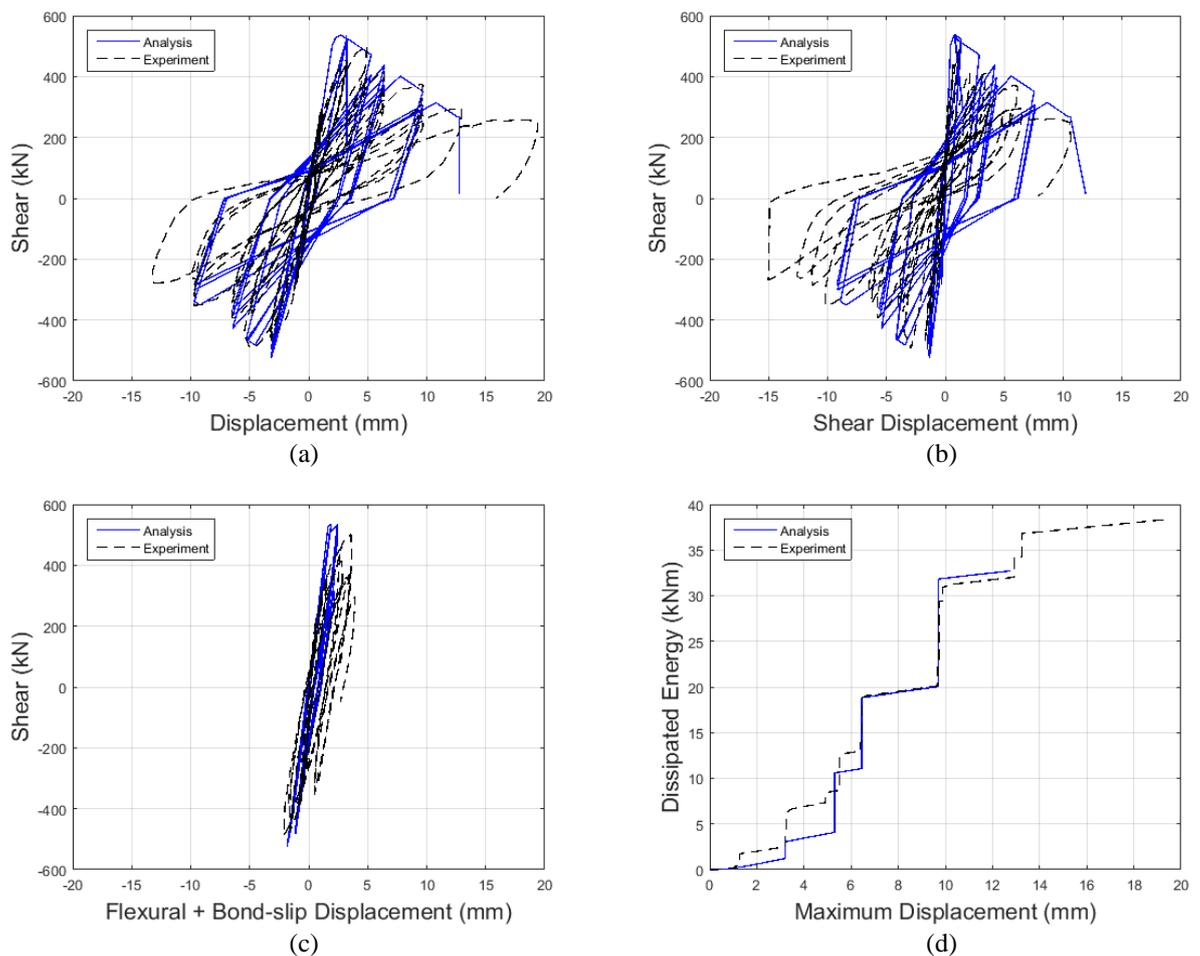
Figure 9-5: Comparison between the predicted response of C-2 by the proposed model and the experimental one in terms of (a) shear force against lateral displacement, (b) shear displacement and (c) flexural and bond-slip displacement; (d) cumulative dissipated energy throughout the experiment.
