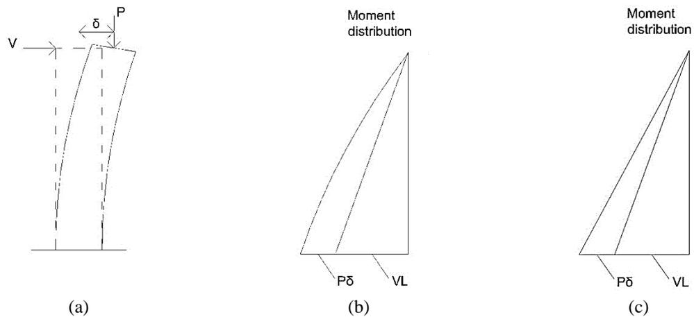
Figure 3-7: (a) Cantilever specimen undergoing constant vertical and cyclic lateral loading; its bending moment distribution (b) following the deflection shape of the specimen, or (c) with linear distribution simplifying assumption.
