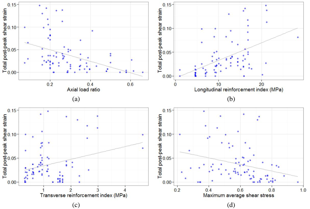
Figure 4-14: Correlation of total post-peak shear strain at the onset of axial failure ( $\gamma_{t,pp}$ ) with (a) axial load ratio based on the capacity of the longitudinal reinforcement,  $v_l$ , (b) longitudinal reinforcement ratio divided by the percentage of confined area,  $\rho_l/\alpha_{conf}$ , (c) transverse reinforcement ratio multiplied by its yield strength,  $\rho_w \times f_{yw}$ , and (d) maximum average shear stress,  $\tau_{max}/\sqrt{f_c}$ .
