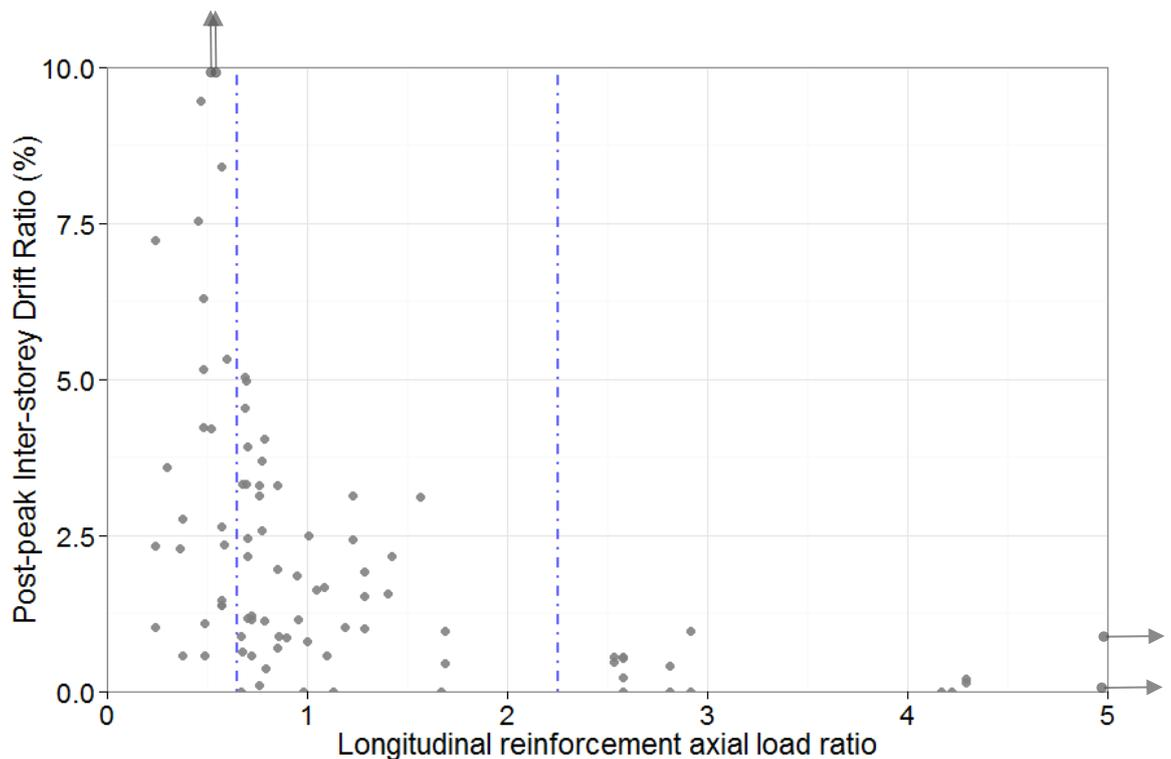
Figure 5-2: Correlation of  $IDR_{pp}$  with the longitudinal reinforcement axial load ratio. Some points are shown with arrows, indicating accurately one of their coordinates and that the other one is higher than the maximum of the range considered on the respective axis.
