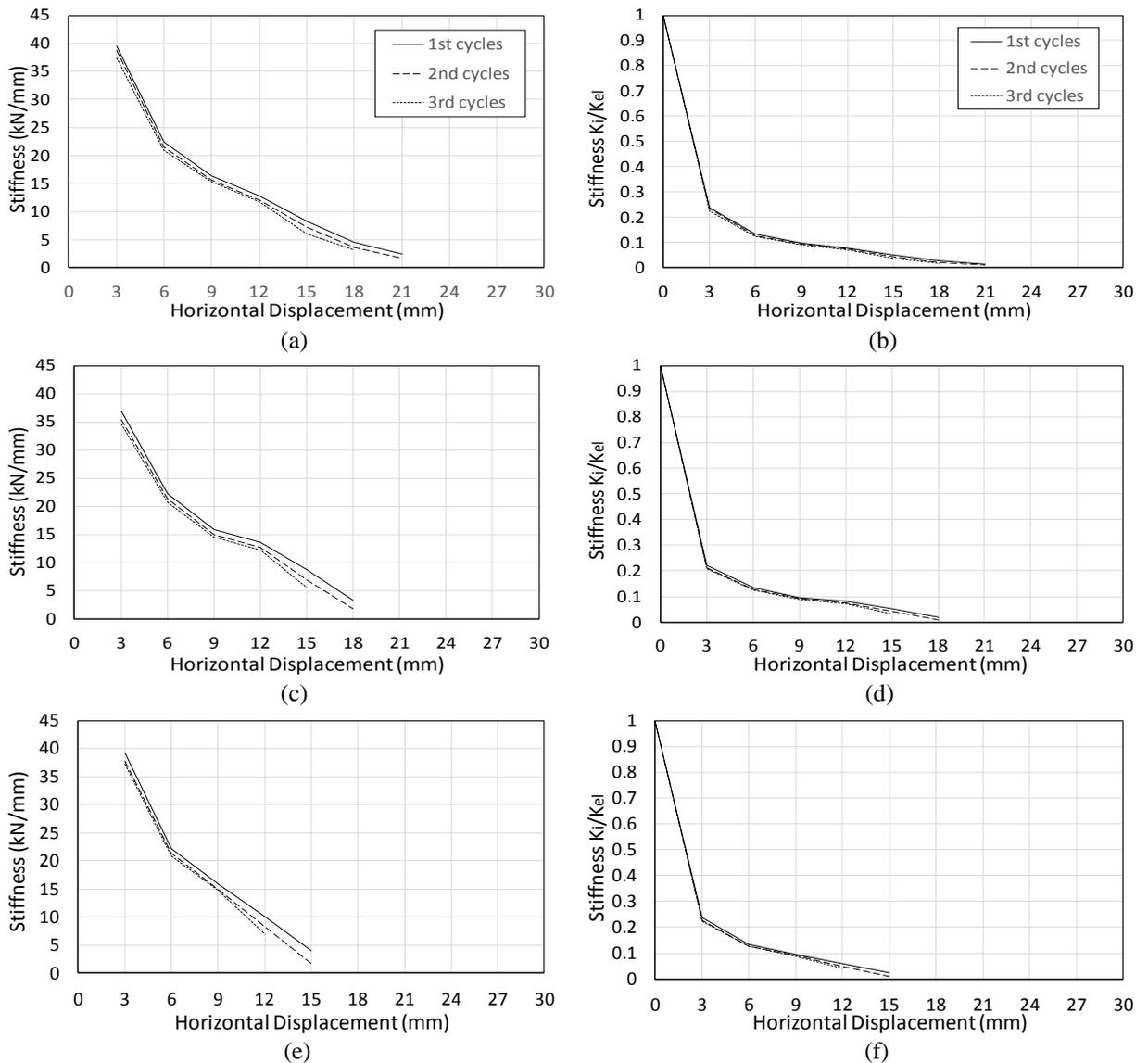
Figure 7-24: Lateral displacement secant stiffness for (a, b) FSC\_1, (c, d) FSC\_2, and (e, f) FSC\_3 in (left) absolute and (right) relative terms.
