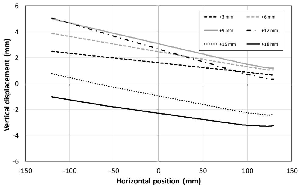
Figure 7-13: Vertical displacement of top of SC\_2 at various displacement level peaks.
