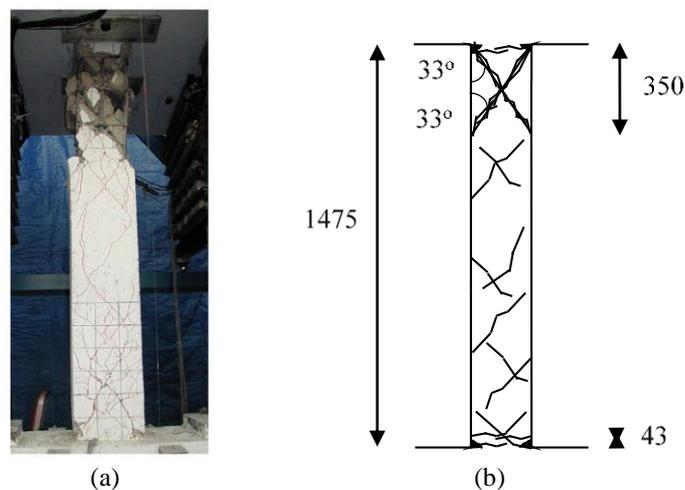
Figure 9-13: (a) Photographic documentation of the damage sustained by Frame 1 (Elwood & Moehle, 2008b); (b) predicted damage by the proposed model.
