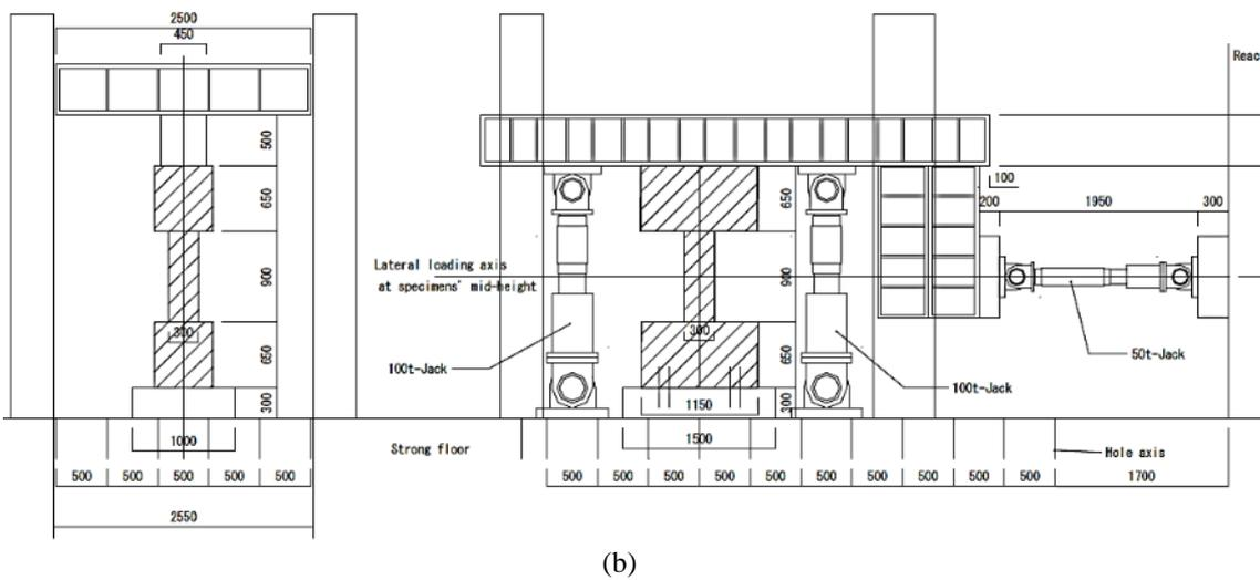
Figure 2-4: (a) Specimen design and (b) test set-up. (Ousalem et al. 2002)
