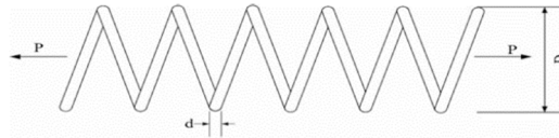
Figure (8.34): A tension/compression spring
