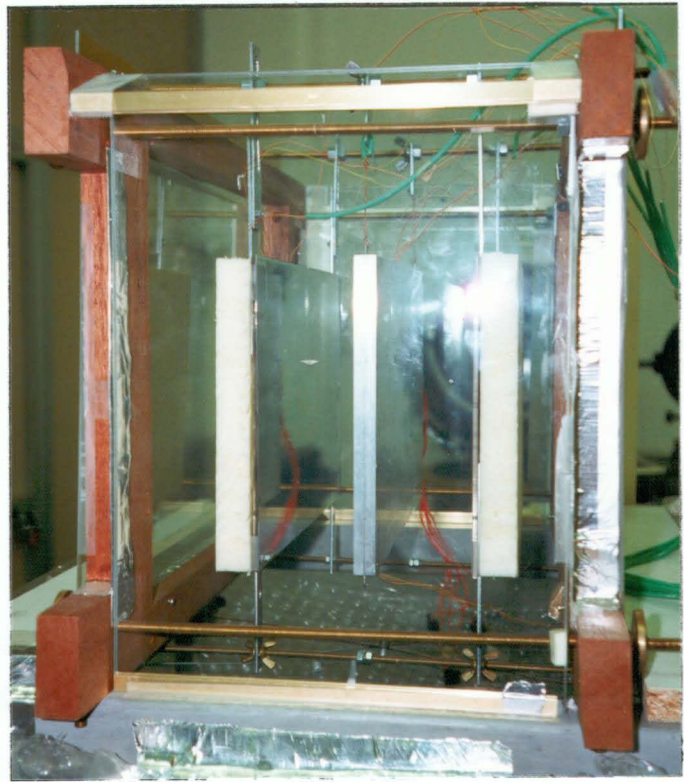
FIGURE 4.9 Sketch and photograph of the smooth channel configuration.
