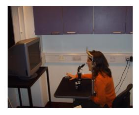
Figure 2.4: Subject positioned at the 0.7 m testing distance.
