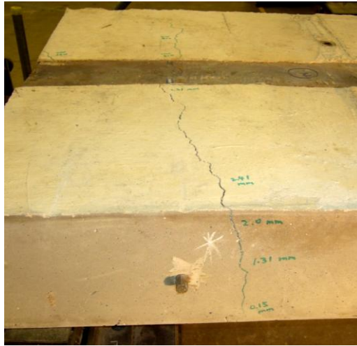
Figure 6.45 Cracks near the support of the shorter shear span
