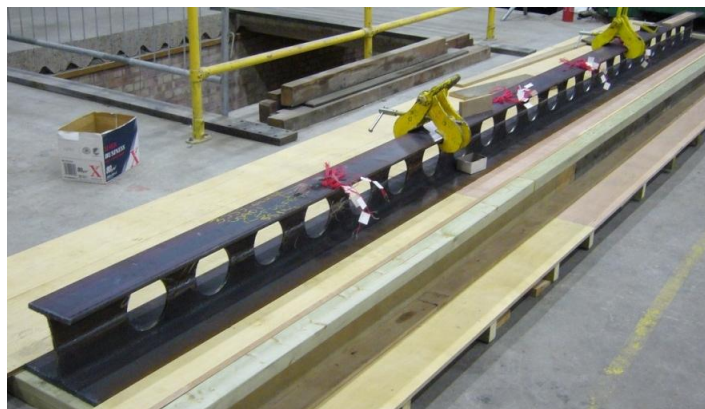
Figure 6.1 Steel section of the composite beam specimen: (a) drawing of cross section, (b) drawing of side view, (c) actual steel section
