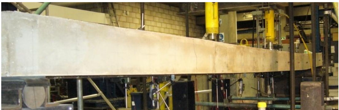
Figure 6.46 Failure profile of the beam specimen in the three-point bending test
