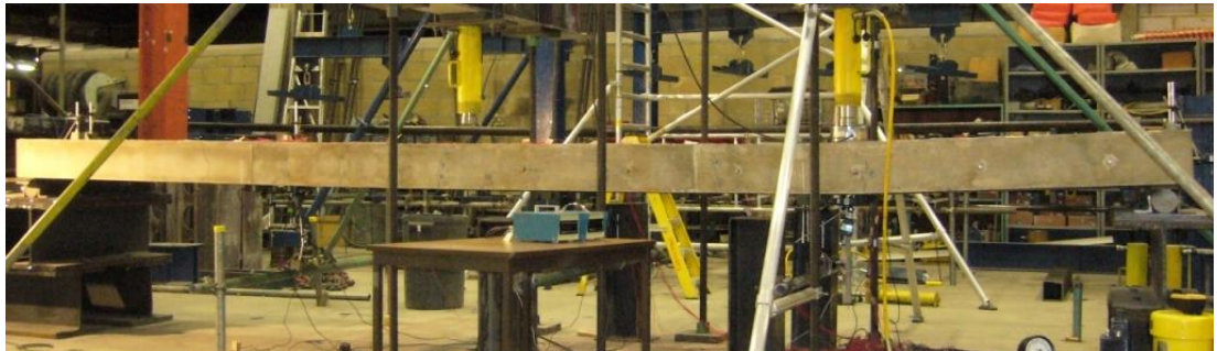
Figure 6.45 Cracks near the support of the shorter shear span
