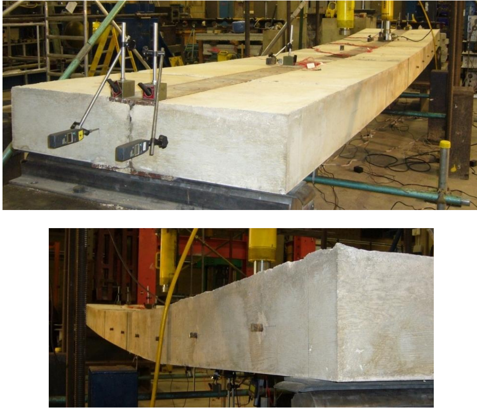
Figure 6.35 Deflected shape of the beam specimen in the three-point bending test
