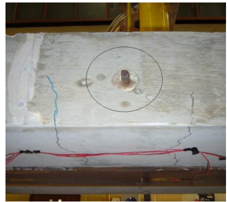
Figure 6.27 Cracking pattern lose to the right loading point
