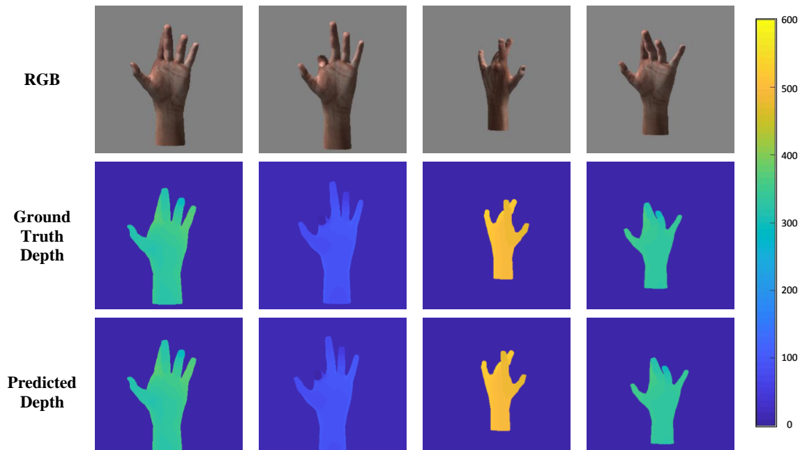
Figure 4.5 Qualitative results using synthetic captured data on four instances of poses. The 1 st row are reference RGB synthetic hand poses. The 2 nd and 3 rd row presents the ground truth and predicted depth as a result of using the proposed method. Observe how almost a perfect recovery was achieved in the synthetic scene.
