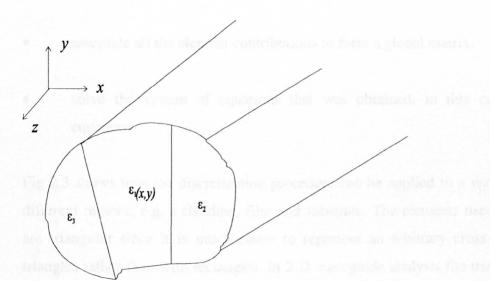
Fig 2.2 Example of an arbitrary shape optical guide with several regions of different material types.
