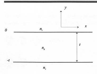
Fig.1.1 Example of a planar waveguide
