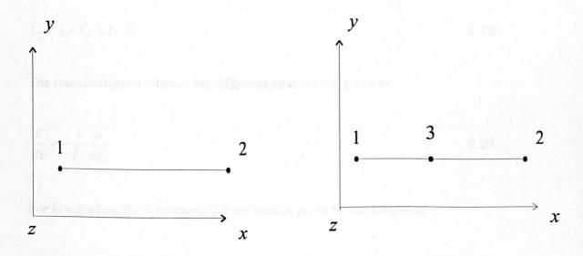
Fig 2.4 Examples of line elements a) Linear element b) Quadratic element.
