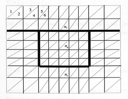
Fig 2.3 Discretization of an optical waveguide
