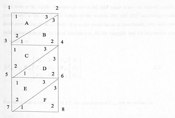
Fig 2.7 Example of domain discretisation using triangular elements
