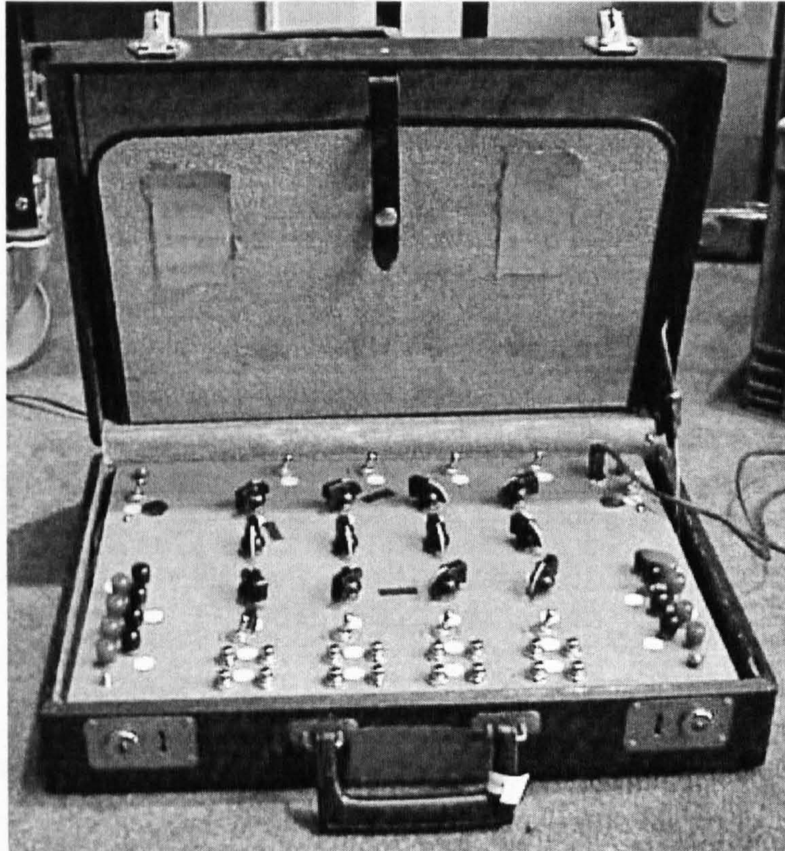
Figure 3-4. Eight channels of low-power amplification built into a briefcase, for performances of Rainforest 1 with the Merce Cunningham Dance Company, circa 1968-1971. This briefcase is seen in the 1971 Rainforest setup in Figure 3-3. Photograph by Matt Rogalsky, 2001.
