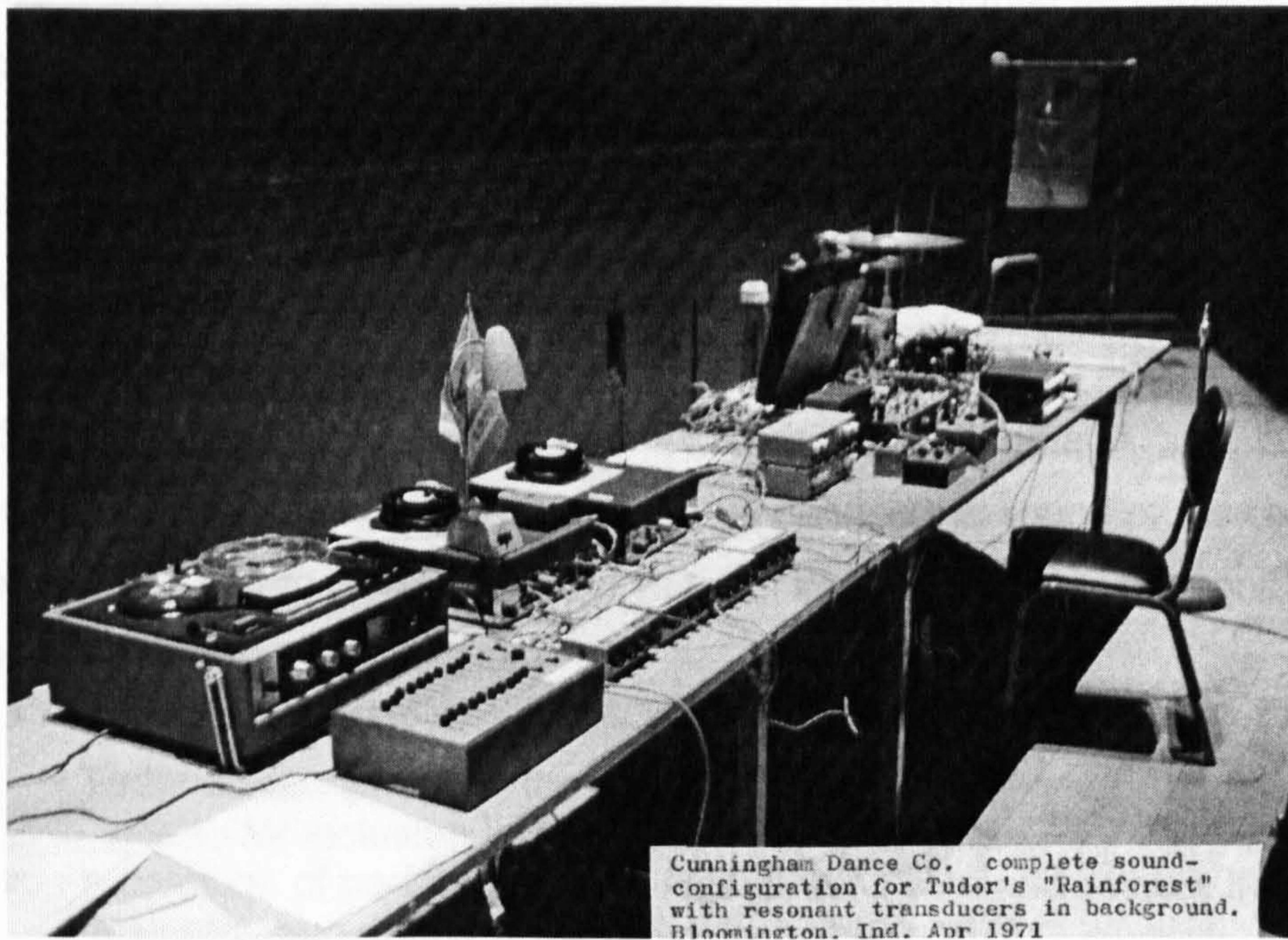
Figure 3-3. A roomy 1971 setup for Rainforest 1 . In the top photograph, two "conventional" signal generators can be seen along with a number of custom-built devices surrounding the eight-channel briefcase amplifier. Transducers can be seen attached to objects (metal sheet, cymbal, and "one of Tudor's glass-enclosed resonating devices of the time" (Mumma 2006a)) in the background of the second photograph. Photographs by Gordon Mumma.
