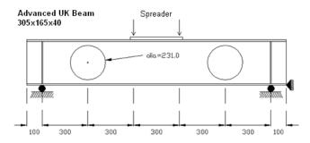
Figure 3. Test specimen configuration.
