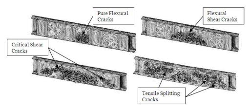
**Figure 5.** Bending and shear crack development at the front side of the beam.
