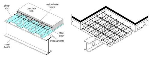
**Figure 1.** Typical composite construction adopted by McGraw-Hill Companies Inc. (left) and Corus (right).
