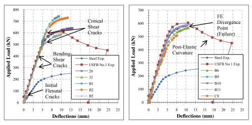
**Figure 4.** Force-deflection curves comparison between experimental test (USFB No.1) and various numerical solutions from "Table 2".
