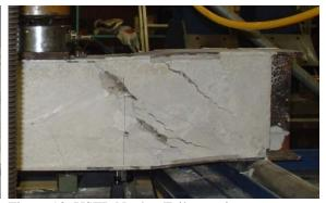
Figure 10. USFB No.4 at Failure point.
