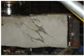
Figure 7. USFB No.1 at Failure point.
