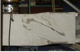
Figure 9. USFB No.3 at Failure point.
