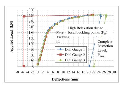
Figure 4: Failure Bare Steel Perforated Section Beam in Flexure.
