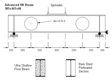
Figure 2. Specimen (all dimensions are in mm).
