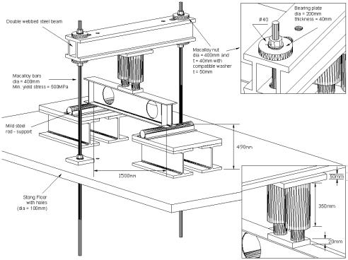
Figure 3. Experimental rig arrangement.
