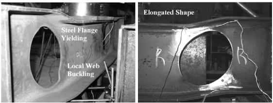
Figure 5. Local highly distorted web - flanges and web opening elongated shape.
