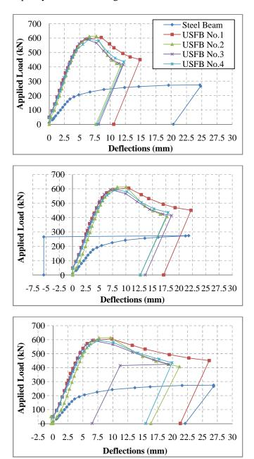
Figure 6. Load vs. Deflection curves for Bare Steel and USFBs for left, middle and right dial gauges.
