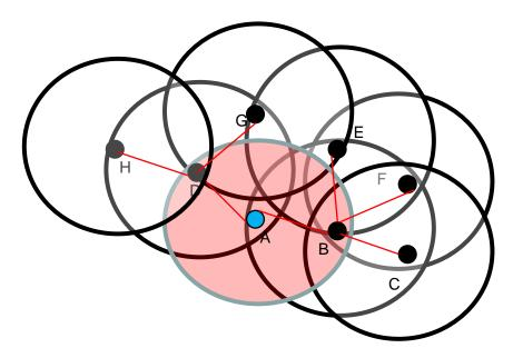
Figure 5-4: Uncovered nodes check the Node ID and rebroadcast clique discovery message with their Node IDs.
