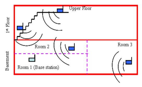
Figure 3-1: Setup for 802.15.4 bit error traces.
