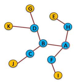
Figure 6-6: Node G, K and J do not receive any Hello message with their node ID as parent ID and therefore consider them as leaf nodes to form the final reduced topology.
