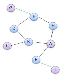
Figure 7-10: Final topology polygon with redundant paths.
