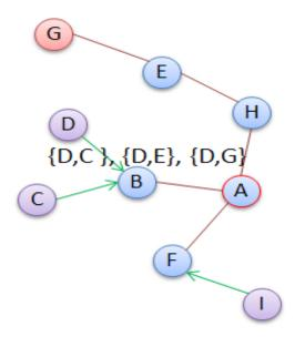
Figure 7-6: Each leaf node sends *finish discovery* message to its parent node and immediate neighbor after the timeout. These sets of nodes are called message paths. Message paths sent by D are shown in the figure.
