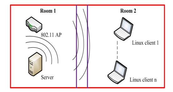
Figure 3-2: Setup for 802.11b bit error traces.
