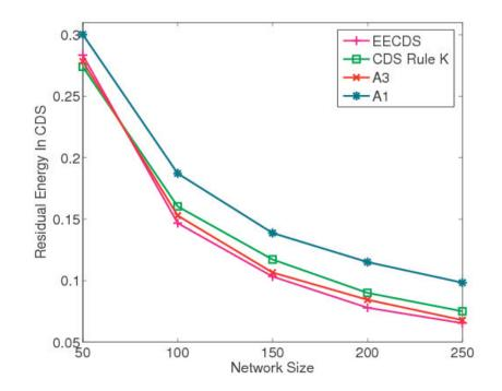
Figure 6-9: Residual Energy under varying network size.
