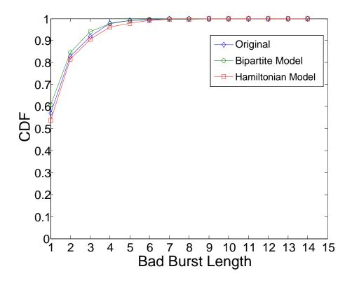
Figure 3-13: Bad burst length distribution for 802.11b bit error traces at K = 8. The CDF for K = 8 is also plotted for good and bad burst lengths and is shown in Figure 3-12 and Figure 3-13. The CDF of the HM clearly follows the CDF of actual
