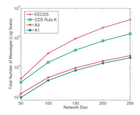
Figure 6-7: Message overhead under varying network size.
