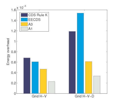
Figure 6-11: Energy overhead under Grid H-V and Grid H-V-D topologies.
