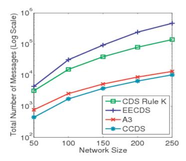
Figure 5-6: Total number of exchanged messaged Vs. Varying node density.
