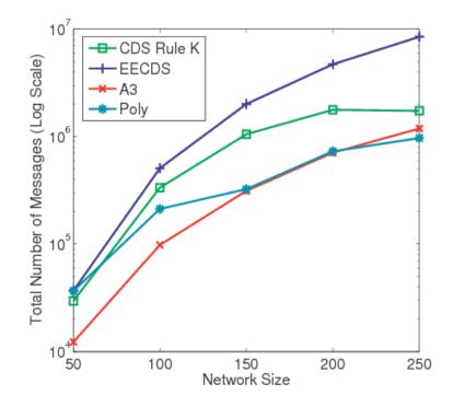
Figure 7-17: Message overhead comparison under dynamic topology maintenance.
