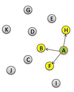
Figure 6-2: Sink node (A) broadcasts Hello message which is received by nodes (B, F and H) under its coverage area. After receiving Hello message, B, F and H
