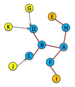
Figure 6-5: Node G and K broadcasts Hello message with parent ID set to node D. Similarly node J broadcasts Hello message with parent ID set to node C.
