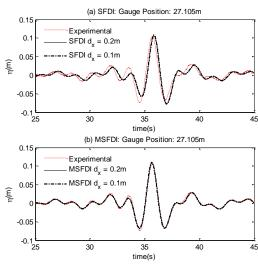
Figure 22: Comparison of the time histories of the wave elevations at x = 27.105m ( $N_l = 1$ ,  $N_z = 20$ )
