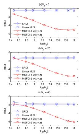
Figure 7: Convergent rate for gradient estimation at free surface particles for  $kh = 10\pi$  (exponential distribution, ka = 0.2,  $N_l = 2$ ,  $\gamma = k$ )
