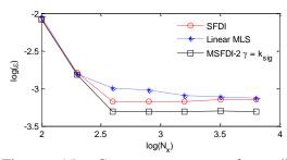
Figure 15: Convergent rate of gradient estimation on the free surface for focusing waves (JONSWAP, peak frequency 0.067Hz, Exponential particle distribution MSFDI-2 with  $N_l = 1$ ,  $N_z = 20$ )
