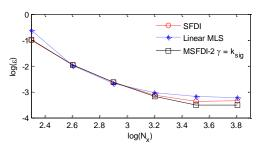
Figure 17: Convergent rate of gradient estimation on the free surface in random sea (JONSWAP, h = 70m, peak period 12.5s,  $H_{I/3} = 12$ m, Exponential particle distribution MSFDI-2 with  $N_l = 1$ ,  $N_z = 20$ )
