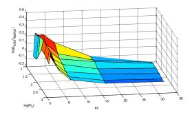
Figure 6:  $\log(\varepsilon_{SFDI}/\varepsilon_{MSFDI})$  for free surface velocity estimations for nonlinear regular waves ka = 0.2 in the cases with different kh(quasi-uniform distribution,  $N_I = 2$ ,  $\gamma = k$ )
