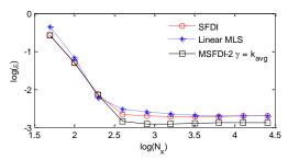
Figure 13: Convergent rate of gradient estimation on the free surface for focusing waves (frequency range  $\sqrt{h/g} \sim 3 \sqrt{h/g}$ , Exponential particle distribution MSFDI-2 with  $N_l=1, N_z=20$ )
