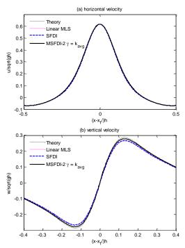
Figure 14: Free surface velocity near the crest at the focusing time (frequency range  $\sqrt{h/g} \sim 3 \sqrt{h/g}$ ; Exponential particle distribution MSFDI-2 with  $N_I = 1$ ,  $N_z = 20$ ,  $N_x = 6400$ )
