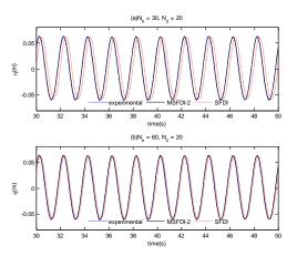
Figure 19: Comparison of the time histories of the wave elevations recorded at the gauge with the experimental data ( $N_1 = 1$ ,  $N_2 = 20$ )
