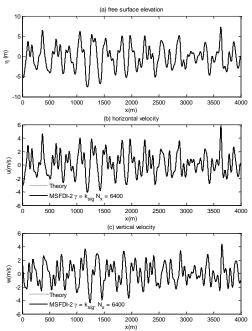
Figure 16: Free surface elevation and velocity in random sea (JONSWAP, h = 70m, peak period 12.5s,  $H_{1/3} = 12$ m, Exponential particle distribution MSFDI-2 with  $N_l = 1$ ,  $N_z = 20$ )
