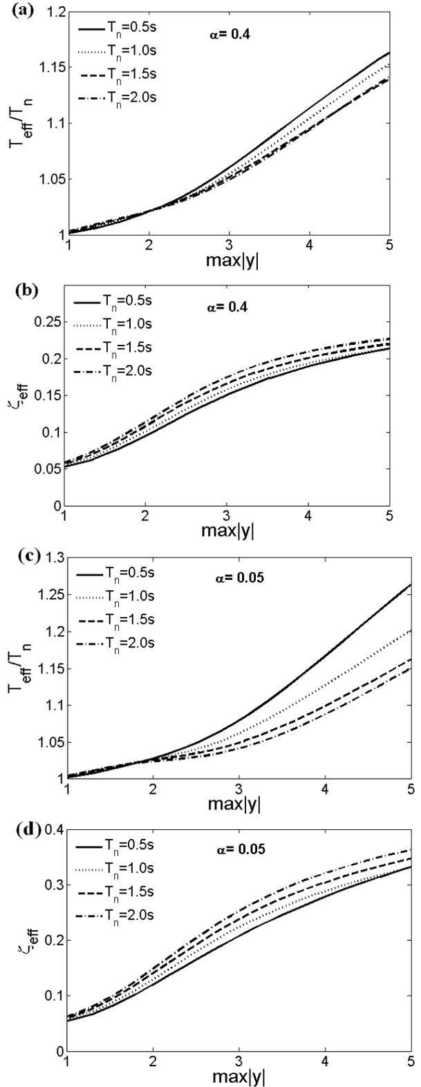
Figure 4. Effective linear properties ( $T_{\text{eff}}$  and  $\zeta_{\text{eff}}$ ) for various bilinear hysteretic oscillators with damping coefficient  $\zeta=5\%$  rigidity ratio  $\alpha$  and pre-yield natural period  $T_n$  compatible with the EC8 spectrum of Figure 2.
