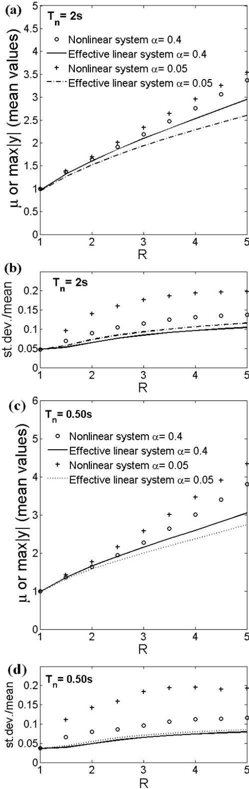
Figure 6. Mean (panels (a) and (c)) and standard deviation over mean (panels (b) and (d)) values of the peak deformation normalized by the yielding displacement  $x_y$  of various bilinear hysteretic oscillators and of the corresponding effective linear systems excited by the suite of accelerograms of Figure 5.
