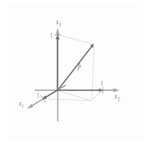
**Figure 4.4:** "Worst" version,  $\bar{P}$ , depicted in terms of the orthogonal basis  $\delta$ . The vector  $\bar{P}$  is a unit vector since its magnitude is 1 (see Eq. (4.9)).
