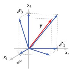
**Figure 6.8:** For a demand space of size 3 there are 2<sup>3</sup> possible "single versions"/"failure regions", including the perfect version represented by the origin, all of which are depicted in this figure. The imperfect single versions are the largest difficulty functions with their associated means, and this is still true in higher finite-dimensions.
