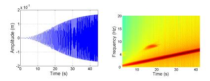
Figure 7.40: Left, fuselage oscillations on the Y axis for  $y_{bl1} = 2.9846$  m,  $y_{bl2} = 2.7846$  m,  $y_{bl3} = 2.8846$  m,  $y_{bl4} = 2.6846$  m. Right, spectrogram of the vibrations shows various frequencies varying between 0 - 7 Hz, 7 - 9 Hz, respectively.
