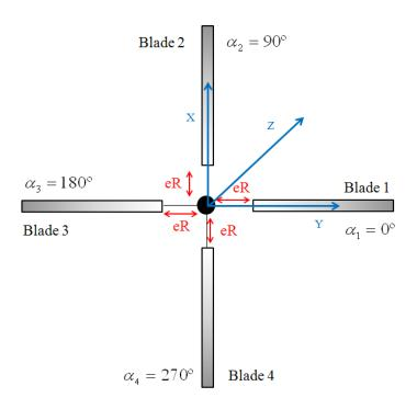
Figure 5.9: Main rotor configuration on nominal position.
