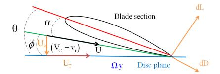
Figure 6.5: Flow conditions in vertical flight for a blade section. This figure is drawn by the author and based on [145].
