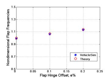
Figure 7.1: Flap frequencies as a function of the offset without flap spring. Red 'o', represents the theoretical predicted values. Blue '\*', VehicleSim obtained values.
