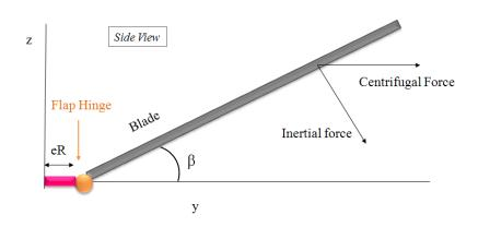
Figure 5.2: Side view of a flap hinge with offset eR.
