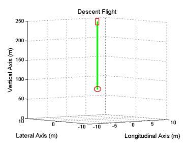
Figure 8.19: Representation in three dimensions in descent flight. Green line shows the helicopter's position. Red ' $\Box$ ', represents the initial position. Red ' $\circ$ ', final position.
