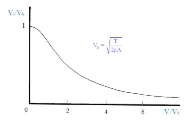
Figure 8.25: Variation of induced velocity with forward speed. This graph is plotted by the author and based on [145].
