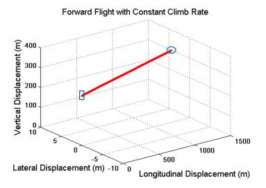
Figure 8.28: Vehicle's position for 50 seconds simulation in which the distance travelled is 994 m with a speed of  $v_{fw} = 20$  m/s and climb rate of 110 m with a speed of 2.2 m/s. Blue ' $\Box$ ', represents the initial position. Blue ' $\circ$ ', final position.
