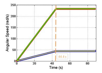
Figure 7.27: Rotor angular speeds. Yellow '-', the main rotor angular speed. Green '-', the tail rotor angular speed. The control signals needed to achieve them are shown on both cases. Blue '\*', the reference signal for the main rotor speed. Red '\*', the reference signal for the tail rotor speed.
