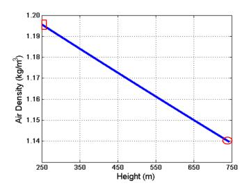
Figure 8.13: Variation of air density in climb flight. Red ' $\Box$ ', represents the starting height. Red ' $\circ$ ', final height.
