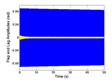
Figure 7.4: Flap amplitude (in blue) and lag amplitude (in yellow) simulation results, showing free vibrations from an initial condition in which the flap angle is  $\beta_0 = 0.09$  rad and lag angle is  $\xi_0 = 0$  rad.
