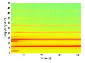
Figure 8.52: Fuselage Y rotation spectrogram when the varying main rotor speed is given by the frequencies:  $f_1 = 7$  Hz,  $f_2 = 0.40$  Hz and  $f_3 = f_1 = 7$  Hz.
