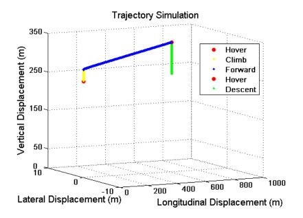
Figure 8.39: Helicopter trajectory.
