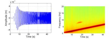
Figure 7.39: Left, fuselage oscillations on the X axis for  $y_{bl1} = 2.9846$  m,  $y_{bl2} = 2.7846$  m,  $y_{bl3} = 2.8846$  m,  $y_{bl4} = 2.6846$  m. Right, spectrogram of the vibrations shows various frequencies varying between 0 - 7 Hz, 7 - 9 Hz, respectively.
