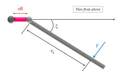
Figure 7.38: Sketch of the force applied on the blade with a lag hinge. This figure is drawn by the author and based on [150].
