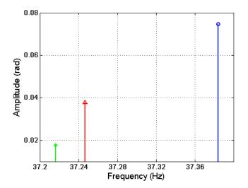
Figure 7.19: Flap frequencies for blade one on the tail rotor. In green '\*', case one. In red ' $\Delta$ ', second case and in blue 'o', results for the third case.
