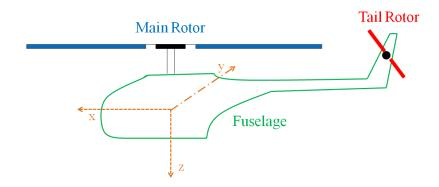
Figure 5.6: Helicopter Sikorsky configuration.
