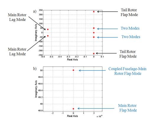
Figure 7.11: a) Root locus for the fuselage, the main and the tail rotors. b) Details of the root locus for two modes.
