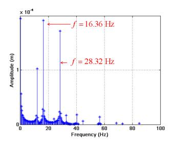
Figure 4.9: Spectrum of vibrations appearing on the fuselage vertical axis.
