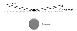
Figure 5.14: Coning angle.
