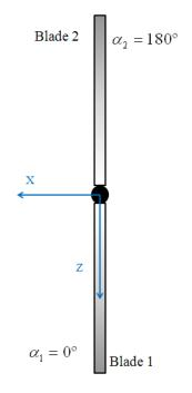
Figure 5.13: Tail rotor nominal configuration.
