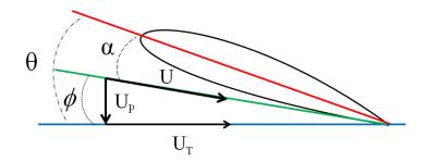
Figure 6.7: Velocity components  $U_T$  and  $U_P$ .
