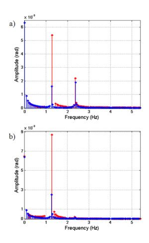
Figure 7.18: a) Fuselage's roll vibrations spectrum. Blue, represents roll vibrations without lag hinge, and red represents roll vibrations with lag hinge included in the model.
