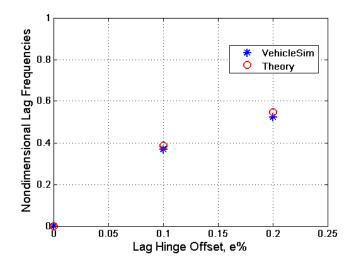
Figure 7.3: Lag frequencies as a function of the offset for the case of no spring, no damper fitted in the lag hinge. Red 'o', represents the theoretical predicted values. Blue '\*', VehicleSim obtained values.
