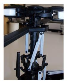
Figure 4.4: Configuration of the swashplate mechanism. Reproduced with permission from Kyosho Corporation.
