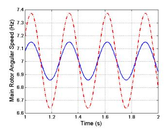
Figure 8.43: Varying main rotor angular speed versus time. Solid blue line represents:  $f_1 = 7 \text{ Hz}, f_2 = 0.16 \text{ Hz}$  and  $f_3 = f_1/2 = 3.5 \text{ Hz}$ . Dotted red line,  $f_1 = 7 \text{ Hz}, f_2 = 0.40 \text{ Hz}$  and  $f_3 = f_1/2 = 3.5 \text{ Hz}$ .
