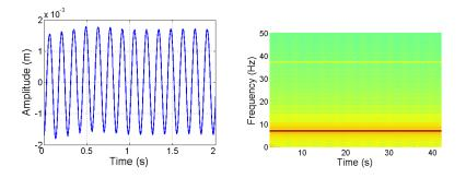
Figure 7.44: Left, fuselage vibrations on the X axis for  $m_{bl1} = 31.06$  kg,  $m_{bl2} = 31.26$  kg,  $m_{bl3} = 29.96$  kg and  $m_{bl4} = 31.16$  kg and  $m_{bltl1} = 6.212$  kg and  $m_{bltl2} = 6.222$  kg. Right, spectrogram of the vibrations shows various frequencies at around 7 Hz and 37 Hz.
