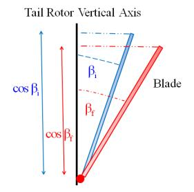
Figure 5.15: The increased cone angle.
