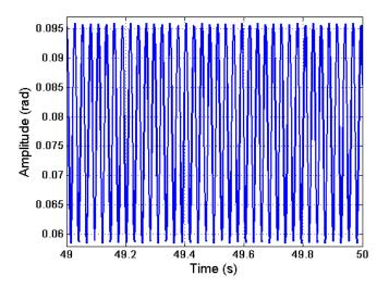
Figure 7.20: First tail rotor blade flap motion. It is worked out with  $a_0 = 0.078$  rad,  $a_1 = 0.017$  rad and  $b_1 = -0.008$  rad. Only time between 49 - 50 seconds is shown in order to clearly see the flap behaviour.
