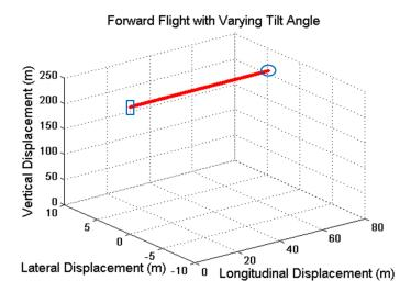
Figure 8.34: Forward flight with varying tilt angle simulation. Red line shows the helicopter's position. Blue ' $\Box$ ', represents the initial position. Blue ' $\circ$ ', final position.
