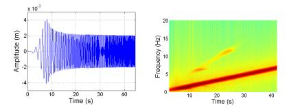
Figure 7.41: Left, fuselage oscillations on the X axis for  $y_{bl1} = 3.9846$  m,  $y_{bl2} = 1.7846$  m,  $y_{bl3} = 3.8846$  m,  $y_{bl4} = 1.6846$  m. Right, spectrogram of the vibrations shows various frequencies varying between 0 - 7 Hz and 6 - 12 Hz.
