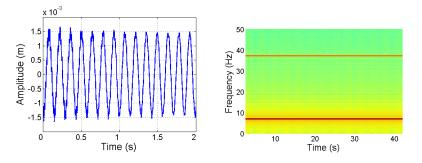
Figure 7.45: Left, fuselage vibrations on the Y axis for  $m_{bl1} = 31.06 \text{ kg}$ ,  $m_{bl2} = 31.26 \text{ kg}$ ,  $m_{bl3} = 29.96 \text{ kg}$  and  $m_{bl4} = 31.16 \text{ kg}$  and  $m_{blt11} = 6.212 \text{ kg}$  and  $m_{blt12} = 6.222 \text{ kg}$ . Right, spectrogram of the vibrations shows various frequencies varying around 7 Hz and 37 Hz.
