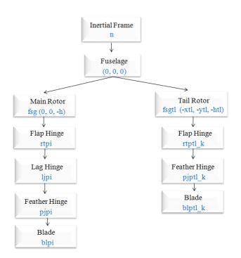
Figure 5.7: Body structure diagram of the Sikorsky model helicopter. Both main and tail rotor in this diagram contain one blade element only due to space restrictions, but the model can contain as many blades as needed.
