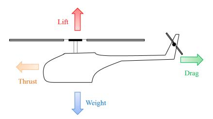
Figure 6.1: Forces acting on a helicopter.
