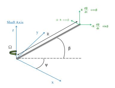
Figure 7.28: Blade flap element velocities, relative to the main rotor axes. This figure is done by the author and based on [150].
