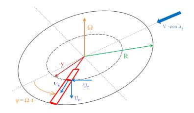
Figure 6.8: Velocity components  $U_T$ ,  $U_P$  and  $U_R$ .
