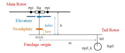
Figure 4.5: Schematic representation of the Caliber 3 VehicleSim model.
