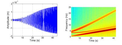
Figure 7.36: Left, fuselage oscillations on the Y axis for eR = 0.982 m. Right, spectrogram of the vibrations shows various frequencies varying between 0 - 7 Hz, 4.5 - 21 Hz and 3.5 - 9 Hz, respectively.
