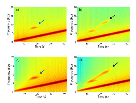
Figure 7.43: a) and c) show the spectrograms for the first simulation when the centre of mass unbalance is given by  $y_{bl1} = 2.9846$  m,  $y_{bl2} = 2.7846$  m,  $y_{bl3} = 2.8846$  m,  $y_{bl4} = 2.6846$  m. b) and d) show the spectrograms for the second simulation when the unbalance is given by  $y_{bl1} = 3.9846$  m,  $y_{bl2} = 1.7846$  m,  $y_{bl3} = 3.8846$  m,  $y_{bl4} = 1.6846$  m.
