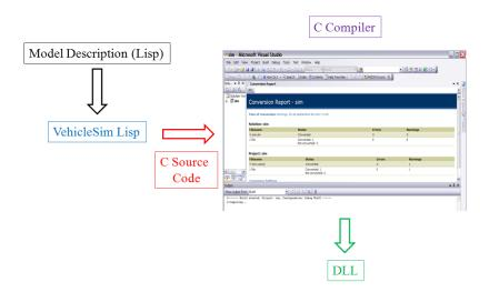
Figure 3.3: Using VehicleSim Lisp to build DLL.
