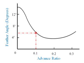
Figure 8.27: Tail rotor feather angle versus advance ratio in forward flight. This graph is plotted by the author and based on [141].
