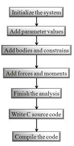
Figure 3.7: VehicleSim commands main sequence. This figure is done by the author and based on [134].
