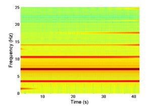
Figure 8.49: Fuselage X rotation spectrogram when the varying main rotor speed is given by the frequencies:  $f_1 = 7$  Hz,  $f_2 = 0.40$  Hz and  $f_3 = f_1/2 = 3.5$  Hz.
