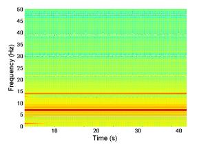
Figure 8.47: Fuselage X position spectrogram when the varying main rotor speed is given by the frequencies:  $f_1 = 7$  Hz,  $f_2 = 0.16$  Hz and  $f_3 = f_1 = 7$  Hz.
