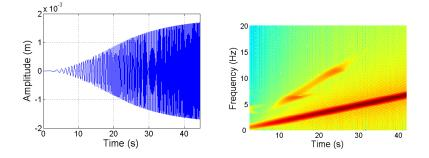
Figure 7.42: Left, fuselage oscillations on the Y axis for  $y_{bl1} = 3.9846$  m,  $y_{bl2} = 1.7846$  m,  $y_{bl3} = 3.8846$  m,  $y_{bl4} = 1.6846$  m. Right, spectrogram of the vibrations shows various frequencies varying between 0 - 7 Hz and 5 - 12 Hz.
