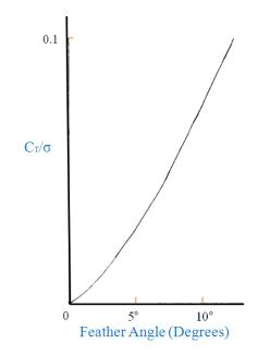
Figure 8.4: Main rotor hover characteristics: thrust coefficient divided by solidity versus feather collective angle. This graph is plotted by the author and based on [145].
