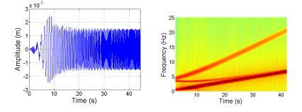
Figure 7.33: Left, fuselage oscillations on the X axis for eR = 0.01 m. Right, spectrogram of the vibrations shows various frequencies varying between 0 - 7 Hz, 4.5 - 21 Hz and 3.5 Hz, respectively.
