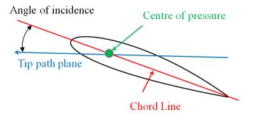
Figure 6.2: Angle of incidence is the angle between the chord line and the tip path plane.
