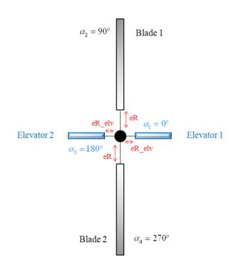
Figure 4.6: Caliber 3 model main rotor nominal configuration.
