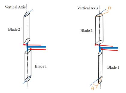
Figure 5.16: Tail rotor blades and the collective angle.
