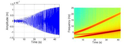
Figure 7.34: Left, fuselage oscillations on the Y axis for eR = 0.01 m. Right, spectrogram of the vibrations shows various frequencies varying between 0 - 7 Hz, 4.5 - 21 Hz and 3.5 Hz, respectively.
