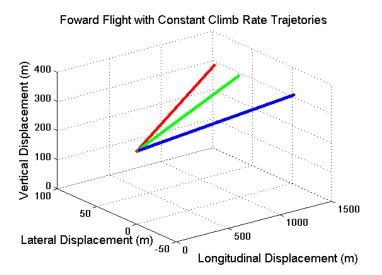
Figure 8.38: Several trajectories in forward flight with constant climb rate and different rates of yaw (ryaw). Red line, represents ryaw = 0.1 rad/s. Green line, ryaw = -0.1 rad/s. Blue line, ryaw = -0.2 rad/s.
