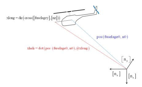
Figure 5.17: Diagram of helicopter's longitudinal position.
