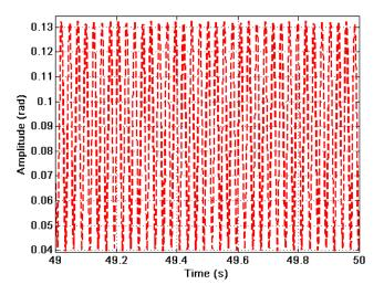
Figure 7.21: First tail rotor blade flap with  $a_0 = 0.087$  rad,  $a_1 = 0.043$  rad and  $b_1 = -0.017$  rad. Only time between 49 - 50 seconds is shown as in the previous figure.
