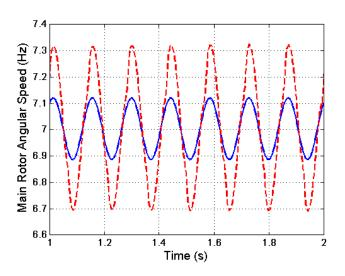
Figure 8.44: Varying main rotor angular speed versus time. Solid blue line represents:  $f_1 = 7 \text{ Hz}, f_2 = 0.16 \text{ Hz} \text{ and } f_3 = f_1$ . Dotted red line,  $f_1 = 7 \text{ Hz}, f_2 = 0.40 \text{ Hz}$  and  $f_3 = f_1$ .
