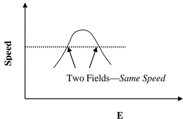
Fig.6. Schematic diagram of charge speed as a function of electric field when a negative differential resistance occurs.
