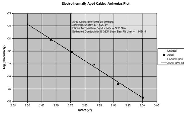
Fig. 5. Arrhenius plot of dc-conductivity in cable section
