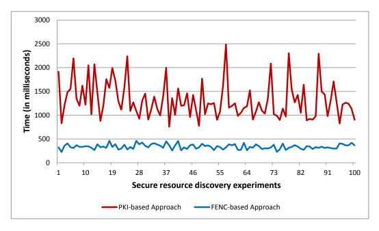
Figure 6.2: Secure resource discovery for 100 runtime trials between PKI and Functional Encryption based approaches in ICVPN, on a single cloud platform
