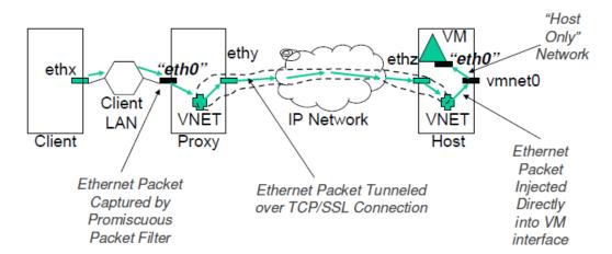
Figure 2.1: Architecture of a VNET based communication framework, showing the establishment of a secure connection between a client and the end host via a *proxy* gateway [146].
