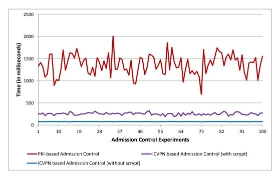
Figure 5.2: Duration of the admission control process for 100 trial instances using the PKI-based and ICVPN methods, between BT and Flexiant cloud platform
