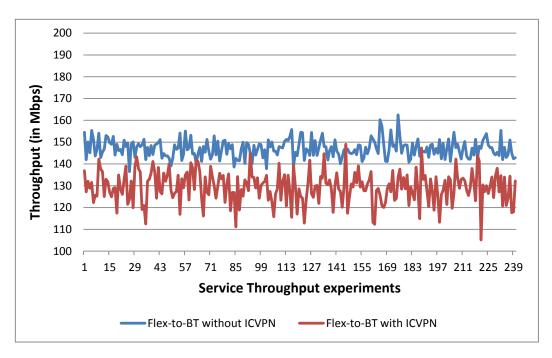
Figure 4.13: Throughput of 240 data transmission experiments *from* Flexiant *to* BT clouds
