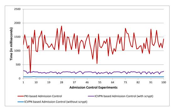
Figure 5.1: Duration of the admission control process for 100 trial instances using the PKI-based and ICVPN methods, on a single cloud platform (BT)
