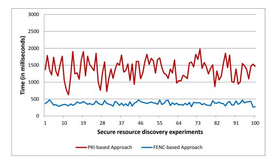
Figure 6.3: Secure resource discovery for 100 runtime trials between PKI and Functional Encryption based approaches in ICVPN, between BT and Flexiant cloud platform
