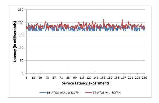
Figure 4.10: Service latency of 240 HTTP HEAD round-trip time request-response messages *from* BT *to* ATOS clouds
