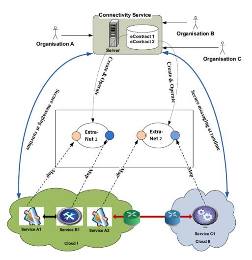
Figure 2.10: Architecture of the eContract-based secure intra-cloud and intercloud connectivity service. The figure shows two extranets formed by the Connectivity Service that offer services from both Cloud I and Cloud II [40]
