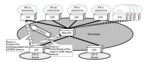
Figure 2.9: Architecture of the hybrid IPsec-VPN model, where the Hub gateway (Hub-GW) is extended using the MOBIKE or Traffic Selector extension in order to perform load-balancing operations [89].
