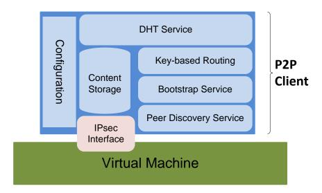
Figure 4.3: Architecture of a Inter-Cloud VPN *P2P Client* node, the architecture being identical for both super peer nodes in the Universal Overlay and VPN peer nodes in a VPN Overlay
