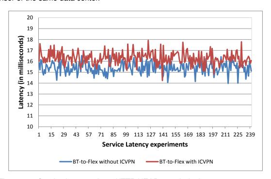
Figure 4.8: Service latency of 240 HTTP HEAD round-trip time request-response messages *from* BT *to* Flexiant clouds
