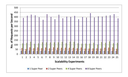
Figure 4.14: Experiments measuring bootstrapping requests processed per second against increasing number of Super Peers
