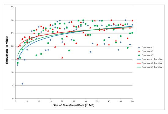
Figure 4.4: Plot of 150 throughput measurements of 1-50 MB data transfers between ATOS and BT cloud platforms in order to find the most stable 3-tuple measurements
