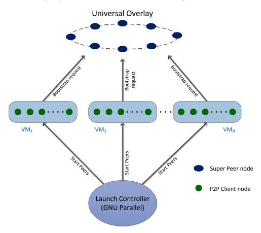
Figure 4.7: Design of the load scalability experiment to measure the effects of increasing the numbers of parallel bootstrapping requests from the VPN peer nodes (P2P Clients) to the Universal Overlay
