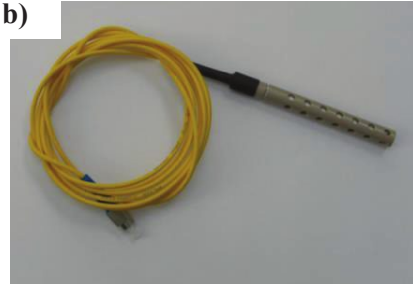
Figure 2. Schematic of the housing (a) and picture of the packaged fibre optic humidity sensor (b).
