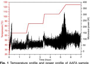
Fig. 1 Temperature profile and power profile of AAFA sample under microwave curing
