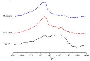
Fig. 3 <sup>29</sup>Si NMR spectra of raw fly ash and AAFA under thermal oven curing and microwave curing
