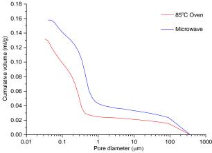
Fig. 4 Pore size distribution of hardened AAFA under thermal oven curing and microwave curing
