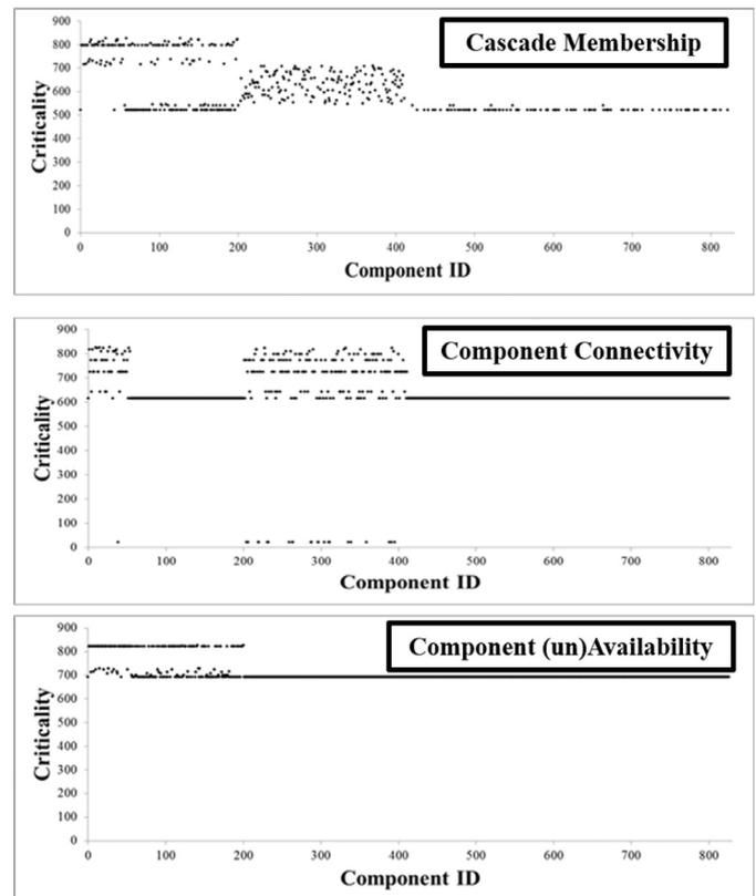
Fig. 8. A comparison of three notions of criticality (with  $\alpha = 1$ ). Each criticality notion results in a ranking of the 829 modelled components. Many of the components in each plot share the same criticality value,<sup>18</sup> resulting in a wide vertical “gap”, in each plot, within which no components assume any criticality values. The size and location of this “gap” differs across the criticality notions.
