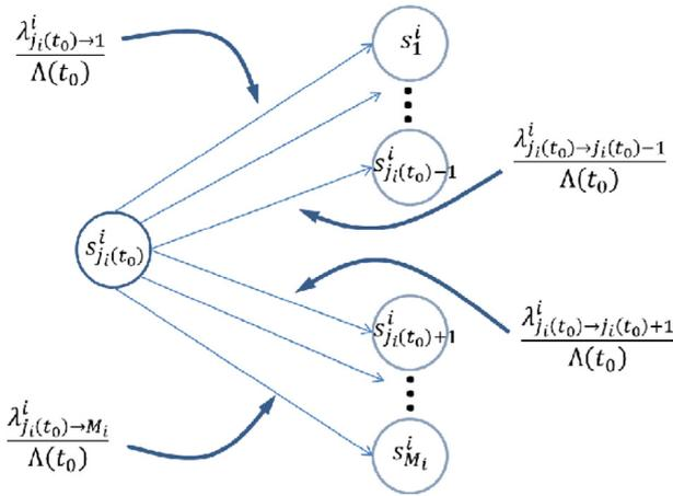
Fig. 3. Using a competing risks algorithm, an ME transits, with probability, from a state  $s_{j_i}^i(t_0)$  at time  $t_0$  to some other state at some future point in time. In this example, each transition’s associated probability of occurrence is a quotient (such as  $\frac{\lambda_{j_i(t_0)-1}^i}{\Lambda(t_0)}$ ) of transition rates for exponential distributions.
