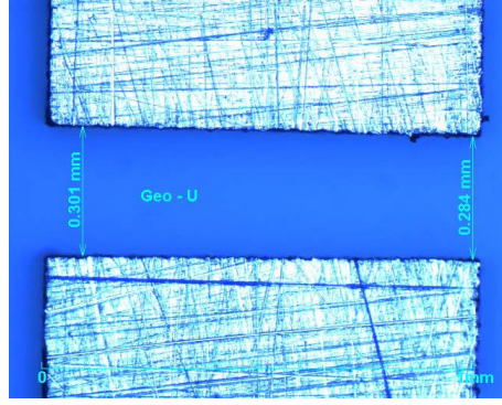
Figure 2.2: Throttle geometry "U" in 300 \mu\text{m} thick sheet steel. 301 \mu\text{m} inlet width, 284 \mu\text{m} outlet width, 20 \mu\text{m} inlet radius, 1 mm throttle hole length. Source: Winklhofer et al. (2001)
