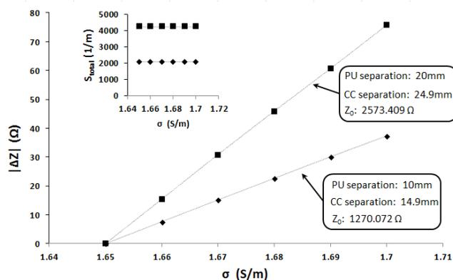
Fig. 5: Simulated change in transfer impedance magnitude for different PU and CC separation, while keeping the PU and CC separation constant, for various conductivities for **Prb2**. Associated change in total sensitivity (embedded plot)
