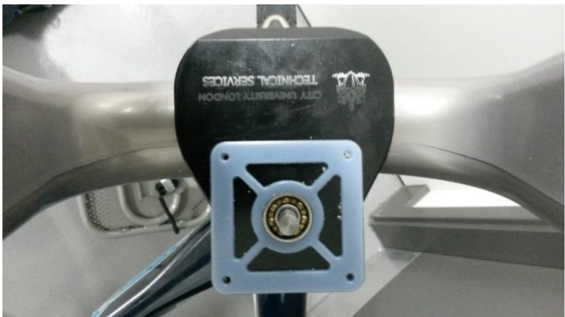
Figure A-10: Plates and shaft installed on the steering hub of the bicycle
