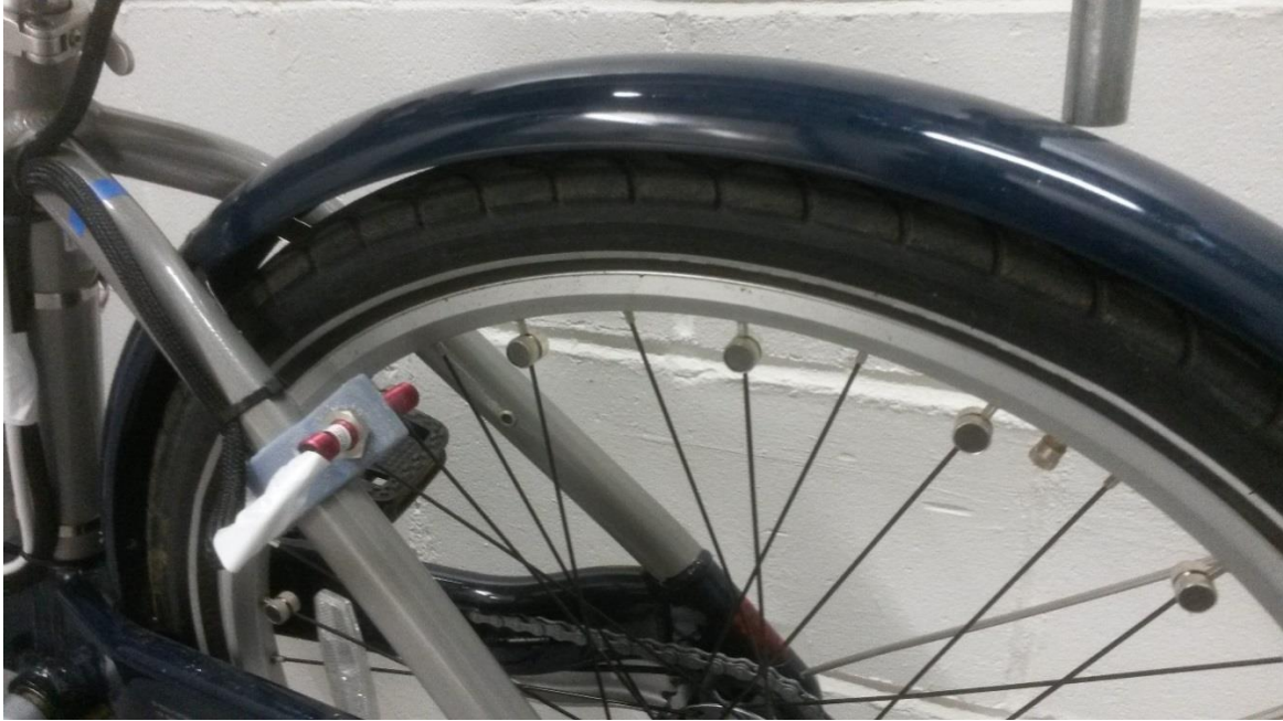
Figure 5-3: Installation of spoke magnets
