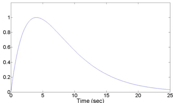
Figure 3. The Bogdanoff-Golberg-Bernard modulating function for  $t_p=4\text{sec}$
