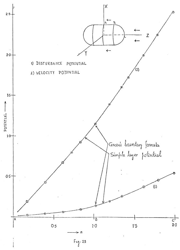
POTENTIALS ON THE SURFACE OF A CYLINDER WITH HEMISPHERICAL CAPS .
