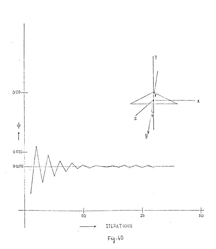
BEHAVIOUR OF THE SOLUTION AT A FIXED POINTP ON SUCCESSIVE ITERATIONS : VALUE OF & AT P IS 0.0372 (INTEGRAL EQUATION METHOD).
