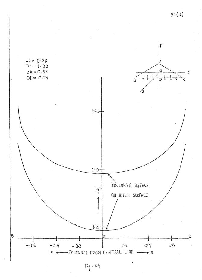
DOWNWARD VELOCITY COMPONENT ON THE UPPER AND ON THE LOWER SURFACES OVER THE LINES Y = CONSTANT (-0.17). (Uz stands for velocity component in z-direction)
