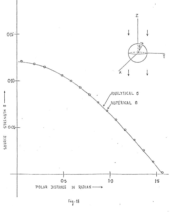
SOURCE DISTRIBUTION ON THE SURFACE OF A SPHERE
