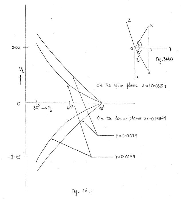
TANGENTIAL COMPONENT OF VELOCITY ALONG THE CIRCULAR ARCS ON THE SURFACES  $Z = \pm H$ NEAR THE TIP OF THE DELTA.
