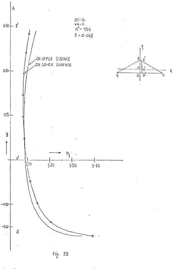
DOWNWARD VELOCITY COMPONENT ON THE UPPER AND ON THE LOWER SURFACES ALONG A LINE X-CONSTANT (0.0208) PASSING THROUGH E<sup>1</sup>C<sup>1</sup>D<sup>1</sup>. DOWNWASH ON THE LINE y = -0.1684 on the surfaces  $z = \pm 0.0481$
