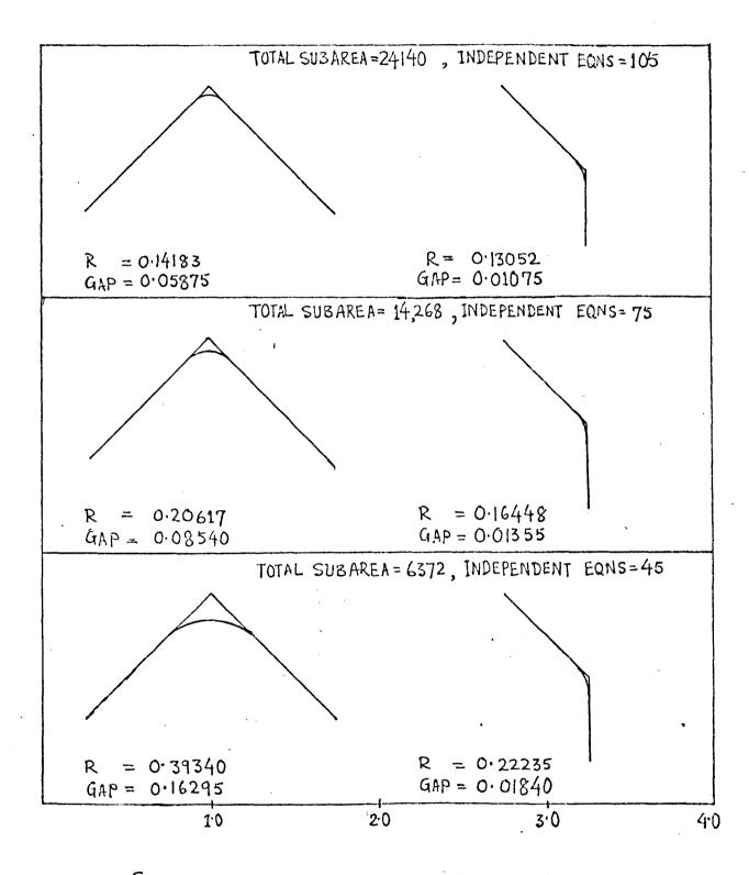
SUCCESSIVE STAGES OF APPROXIMATIONS OF THE CONE AT THE TOP AND THE CORNER AT THE EDGE  $\cdot$ R = RADIUS OF CURVATURE
