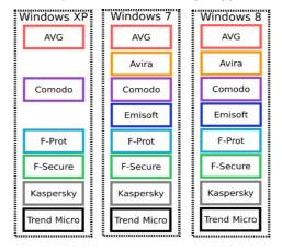
**Figure 5-1** The AV products and OSs currently supported in AVAMAT. Each box is one virtual machine (we refer to a box as VM(a,o)). Avira and Emisoft no longer support Windows XP versions, hence they are missing from the figure above :Windows XP on left-side of box.
