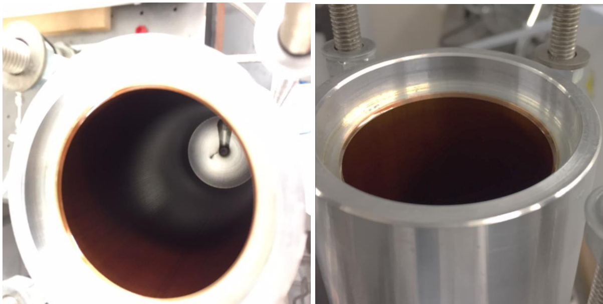
Figure 10.2 Photographs of fuel receiving cylinder with its internal surface coated in a hard-brown lacquer with a polymeric appearance.
