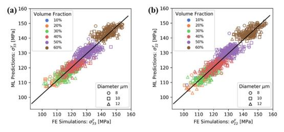
**Figure 6.** Comparisons of the predictions of FE simulations and those of the proposed machine learning approach, for the transverse yield strengths of the composite.
