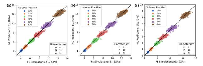
**Figure 5.** Comparisons of the predictions of FE simulations and those of the proposed machine learning approach, for the elastic properties of the material.
