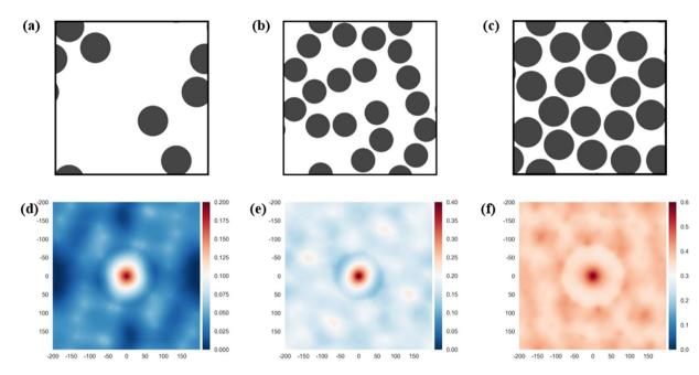
**Figure 1.** Top: example of SVEs with different fibre volume fractions and radii. Bottom: corresponding contours of the 2-point correlation function  $f_r^{FF}$ . (**a,d**):  $\phi_f = 0.2$ ;  $R_f = 5 \mu m$ ; (**b,e**):  $\phi_f = 0.4$ ;  $R_f = 4 \mu m$ ; (**c,f**)  $\phi_f = 0.6$ ;  $R_f = 5 \mu m$ . The labels on the axes of (**d-f**) refer to the number of pixels.
