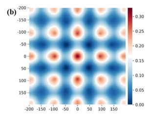
**Figure 7.** (a) Example of a square periodic microstructure with 16 fibres ( $\phi_f = 0.33$ ); (b) Contours of the corresponding 2-point correlation function; the labels on the axes refer to the number of pixels.
