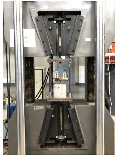
Fig. 7 Pull-out experimental installation
