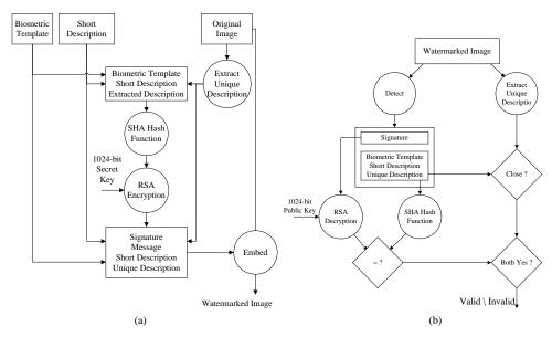
Fig. 1. Cryptographic Encoder / Decoder
