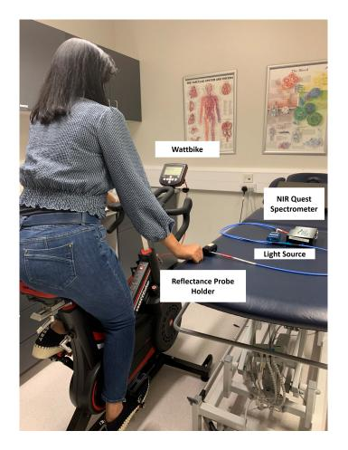
**Figure 9.1:** Set-up of the in-vivo experiments where a volunteer was recruited for an incremental exercise bike study and NIR spectra was collected from the thumb using a portable NIR spectrometer, NIR Quest, a light source and a reflectance probe holder.
