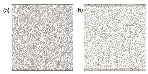
Figure 5.2 (a) grid used in the parametric study, (b) coarser grid.
