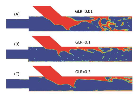
Figure 5.13 Contour of volume fraction of air-water multiphase flow at three different GLRs.
