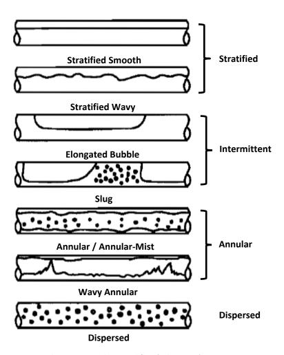
Figure 3.6 Flow patterns in horizontal flow (Baker, 1954).
