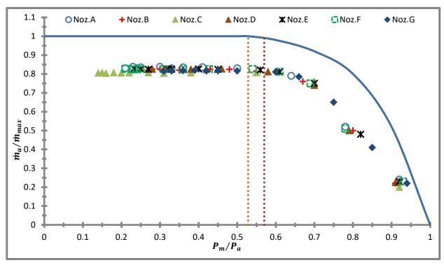
**Figure 5.8** Plot of the ratio of air mass flow rate to maximum air mass flow rate through gas port against pressure ratio. The continuous blue line is the curve for isentropic flow through converging-diverging nozzle.
