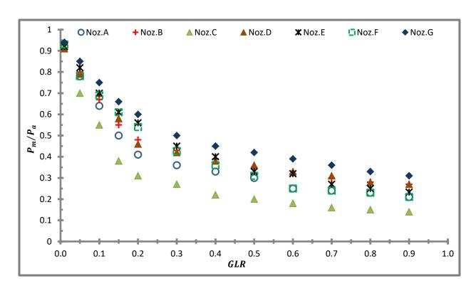
Figure 5.6 Plot of mixing point pressure to air inlet pressure ratio against gas to liquid mass flow rate ratio.
