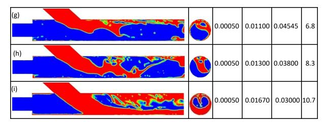
Figure 6.6 Internal flow pattern within the mixing port of internally mixing twin-fluid Y-jet atomizer at the flow time of 0.001 s for the liquid-to-gas momentum ratios of (a) 4.6, (b) 7.3, (c) 8.1, (d) 9.4, (e) 3.2, (f) 5.4, (g) 6.8, (h) 8.3 and (i) 10.7.
