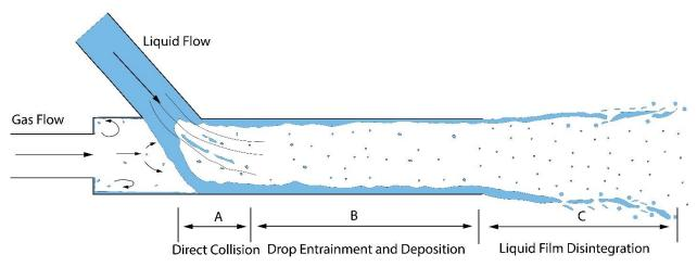
Figure 3.3 Schematic of atomization mechanism in Y-jet atomizer proposed by Song & Lee (Song & Lee, 1996).
