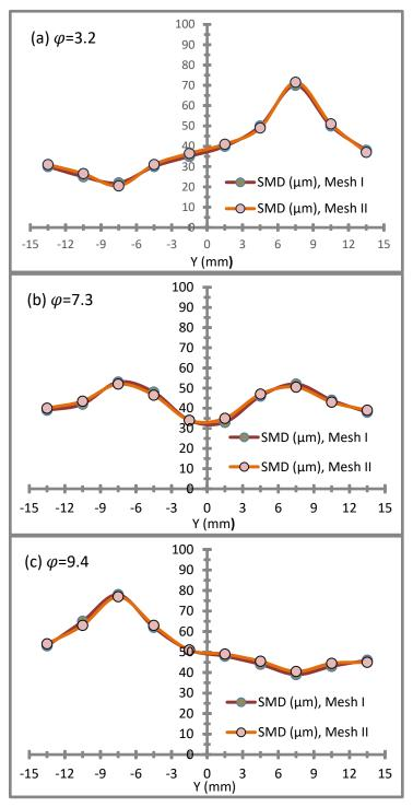
**Figure 6.3** SMD drop size distribution for Mesh I and Mesh II for liquid-to-gas momentum ratios of (a) 3.2, (b) 7.3 and (c) 9.4.
