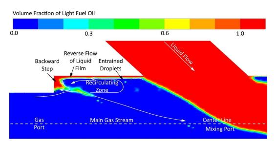
Figure 6.8 illustration of the recirculation in the premix zone of the internally mixing twin-fluid Y-jet atomizer.
