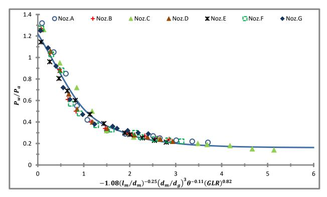
Figure 5.10 Comparison of numerical data points against empirical correlation (eq. 2.4) for the water inlet pressure to the air inlet pressure ratio proposed by Pacifico & Yanagihara (Pacifico & Yanagihara, 2014).
