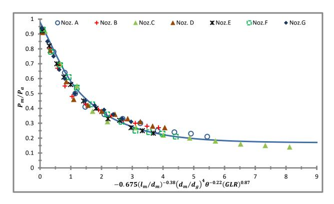
Figure 5.9 Comparison of numerical data points against empirical correlation (Eq. 2.3) for the mixing point pressure to the air inlet pressure ratio proposed by Pacifico & Yanagihara (Pacifico & Yanagihara, 2014).
