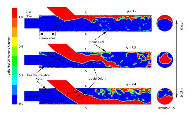
Figure 6.7 illustration of internal flow pattern based on liquid-to-gas momentum ratio.
