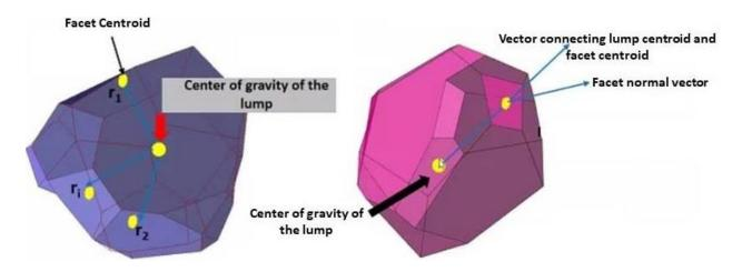
Figure 4.1 Asphericity calculation methods: (a) Normalized radius standard deviation (b) Average radius-surface orthogonality (Courtesy ANSYS Germany).
