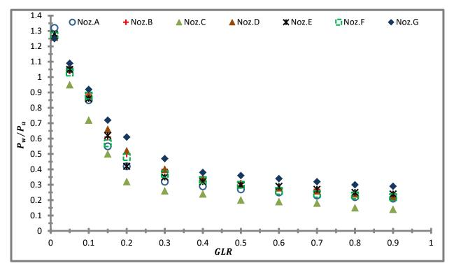
Figure 5.7 Plot of water inlet pressure to air inlet pressure ratio against gas to liquid mass flow rate ratio.
