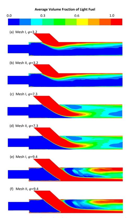
**Figure 6.4** Average volume fraction of light fuel oil over one hundred thousand time steps for liquid-to-gas momentum ratios of 3.2 (a) Mesh I and (b) Mesh II, 7.3 (c) Mesh I and (d) Mesh II, and 9.4 (e) Mesh I and (f) Mesh II.
