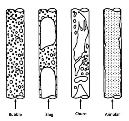
Figure 3.5 Flow pattern in vertical flow (Oshinowo, 1974).
