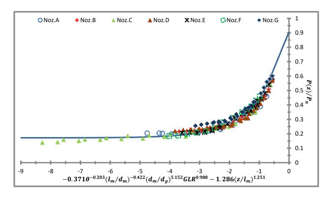
Figure 5.11 Comparison of numerical data points against the empirical correlation (Eq. 2.5) based on GLR for the pressure drop along the length of the mixing port proposed by Pacifico & Yanagihara (Pacifico & Yanagihara, 2014).
