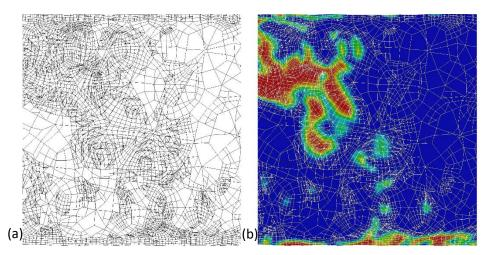
Figure 6.2 (a) Instantaneous grid (b) Instantaneous grid with the superimposed volume fraction of the Light Fuel Oil.
