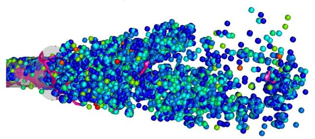
**Figure 6.9** Spray formation by internally mixing twin-fluid Y-jet atomizer at the flow time of 0.0006 s for the liquid-to-gas momentum ratio of 7.3. The magenta colored blobs and ligaments represent the liquid resolved by VOF formulations and spherical particle represents the liquid droplets tracked by DPM model.
