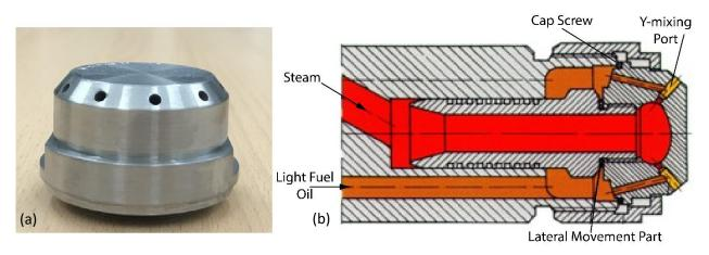
Figure 2.2 (a) nozzle head of twin-fluid Y-jet atomizer (b) Schematic of internally mixing twin-fluid Y-jet atomizer (courtesy MHPS).
