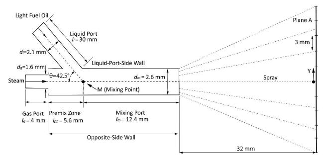
Figure 6.1 Geometry of twin-fluid Y-jet atomizer used in the simulations and schematic explanation of the subsequent spray formation.
