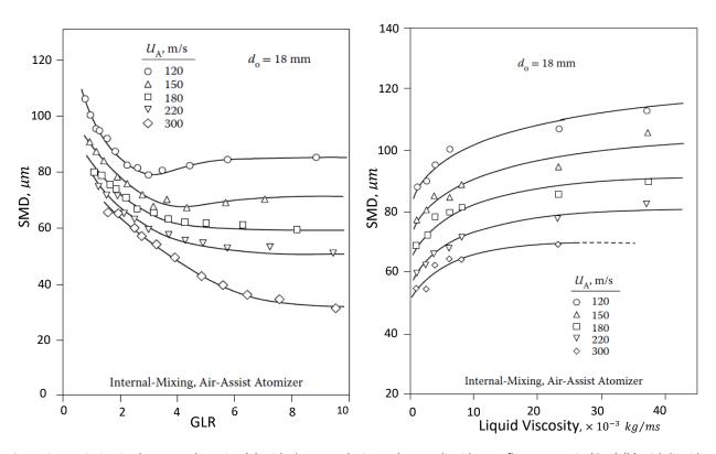
Figure 3.4 Variation in the mean drop size (a) with the gas velocity and gas to liquid mass flow rate ratio (GLR) (b) with liquid viscosity (Inamura & Nagai, 1985).
