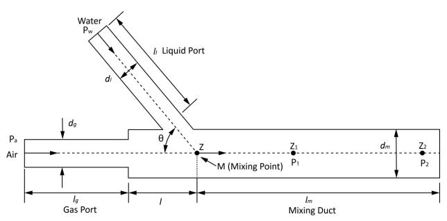
Figure 5.1 Schematic of the nozzle used for the parametric study.
