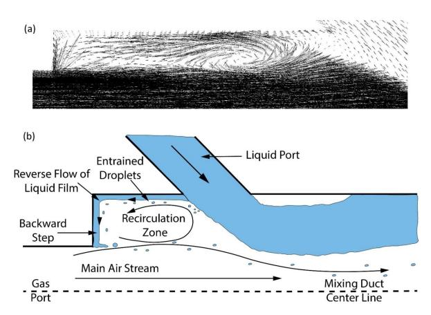
Figure 5.5 (a) recirculating velocity vectors in recirculation zone, (b) schematic illustration of recirculating air flow and reverse film formation.
