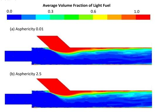
Figure 6.5 Average volume fraction of light fuel oil over 1000 time steps for asphericity ratios of (a) 0.01, and (b) 2.5 for the liquid-to-gas momentum ratio of 2.8.
