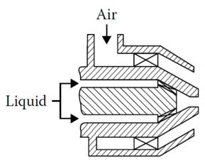
Figure 3.1 External mixing air-assist atomizer.
