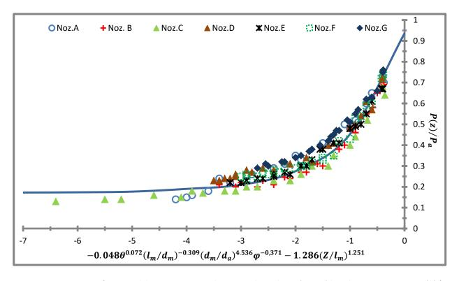
Figure 5.12 Comparison of numerical data points against the empirical correlation (Eq. 2.6) based on momentum ratio ( $\phi$ ) for the pressure drop along the length of the mixing port proposed by Pacifico & Yanagihara (Pacifico & Yanagihara, 2014).
