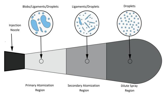
Figure 1.2 A schematic of a liquid spray.
