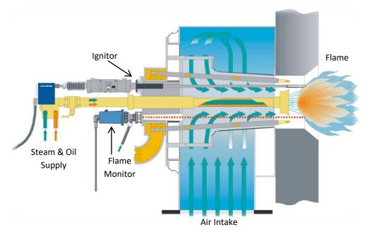
Figure 1.1 Schematic of industrial oil burner (courtesy MHPS).
